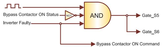
Fig. 7. The operational logic for bypass switch components.
