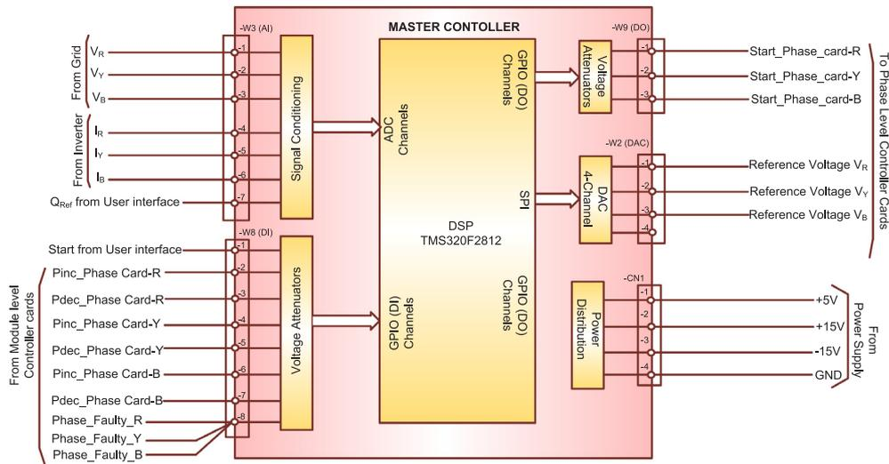
Fig. 14. Signal Exchange diagram of Master controller card.
