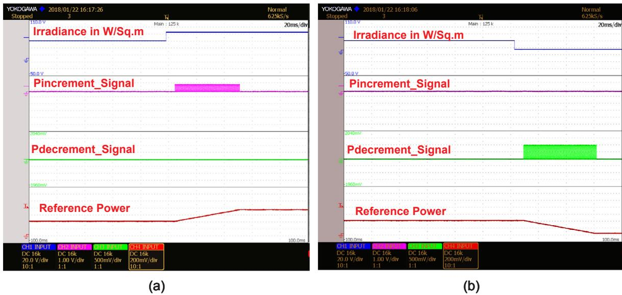
Fig. 16. (a) Increment/Decrement power reference Signals and the reference power during increment in the Irradiance input of PV array. (b) Increment/Decrement power reference Signals and the reference power during decrement in the Irradiance input of PV array.
