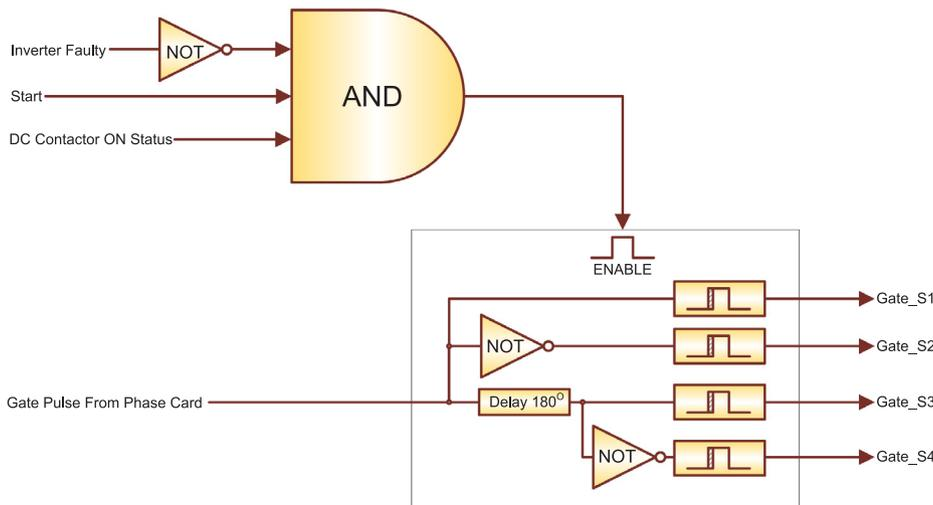
Fig. 6. The operational logic for IGBT Gate pulse distribution in Module-Level Control card.
