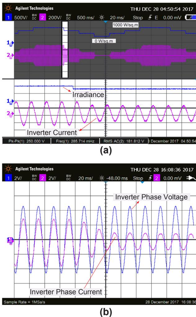
Fig. 24. Transient response of inverter current with change in Irradiance value.
