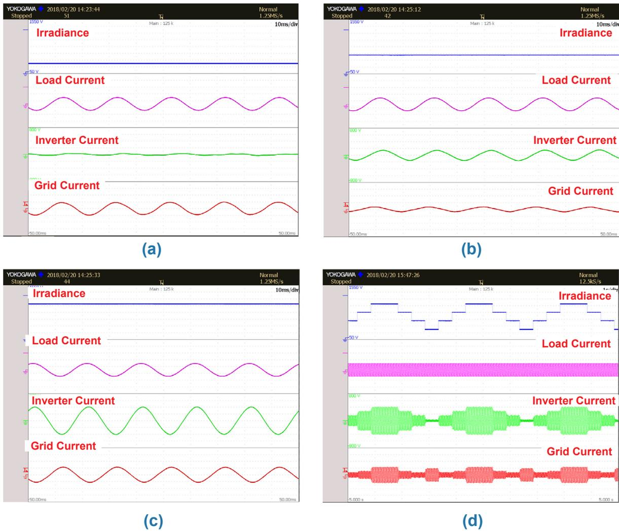
Fig. 22. (a) Load Current, Inverter current and Grid current when irradiance is Zero W/sq m. (b) Load Current, Inverter current and Grid current when irradiance is 250 W/sq m. (c) Load Current, Inverter current and Grid current when irradiance is 750 W/sq m. (d) Steady-state Load Current, Inverter current, and Grid current for different values of irradiance.
