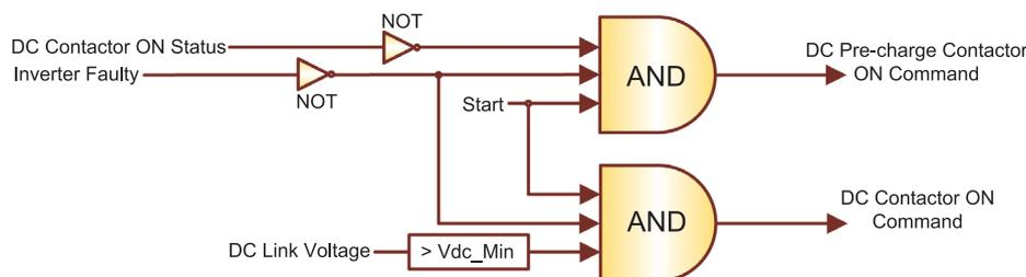
Fig. 4. The operational logic for Pre-charge and main DC Contactors.
