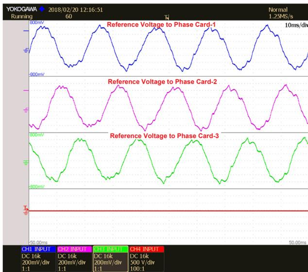
Fig. 23. Reference voltages generated Master Controller Card for Three Phase controller cards.
