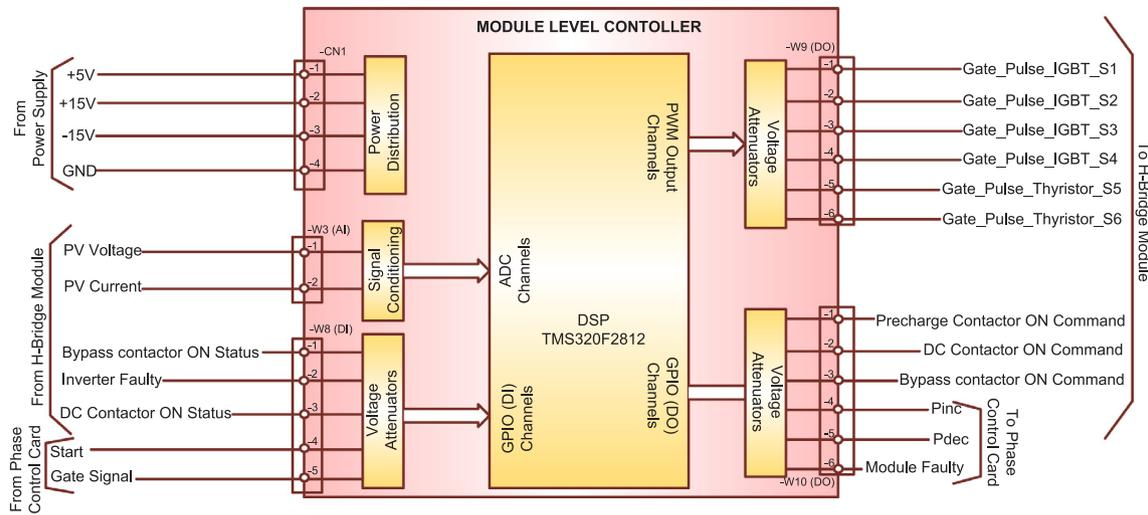
Fig. 8. Signal Exchange diagram of Module level control card.
