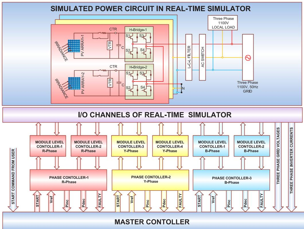
Fig. 21. Block diagram of Controller-In-Loop simulation validation of Master controller card.
