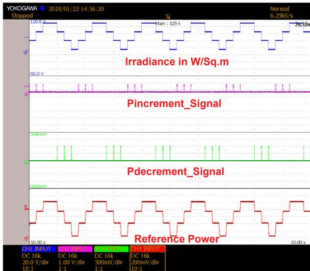
Fig. 17. Increment/Decrement power reference Signals and the reference power during step-change in the Irradiance input of PV array.
