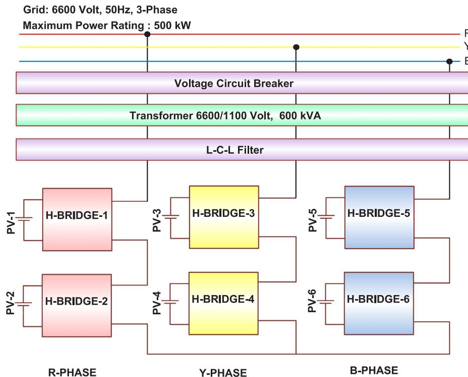
Fig. 2. CHB based PV-Inverter for Grid Connected System.
