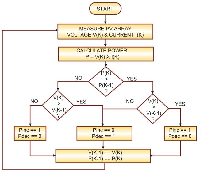
Fig. 5. The operational logic for Perturbation & Observation Method of Maximum power point tracking.
