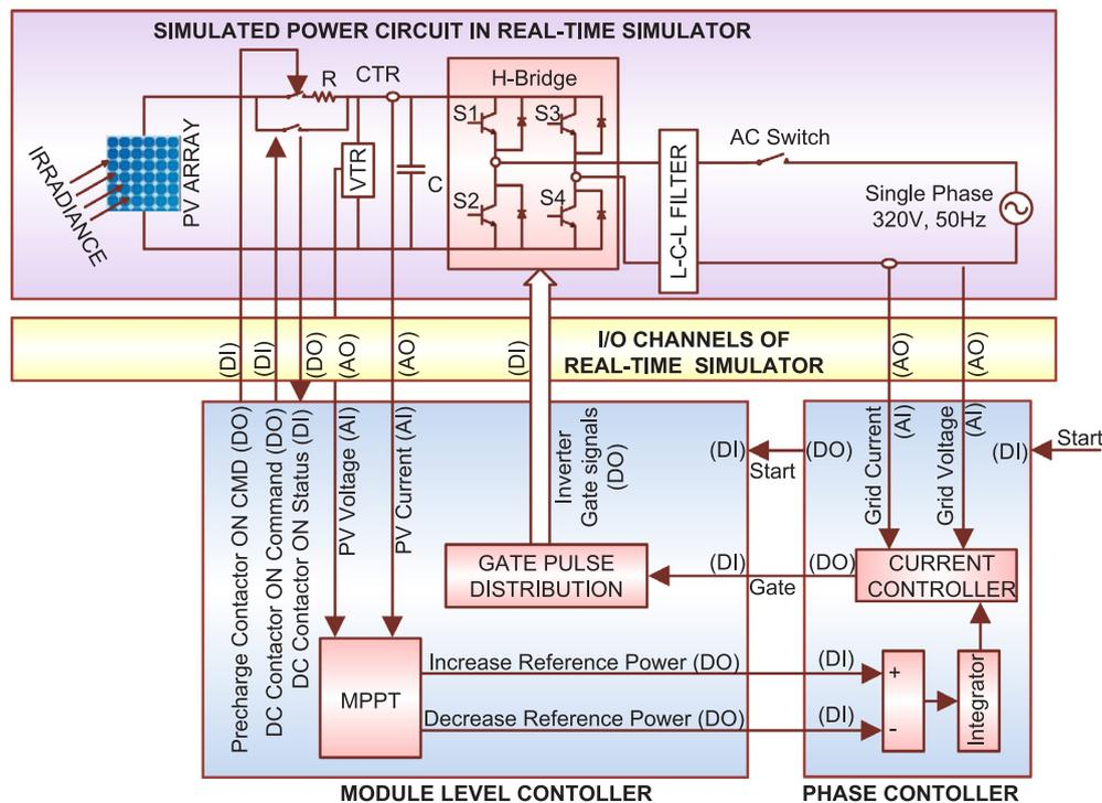
Fig. 15. Block diagram of Controller-In-Loop simulation validation of module-level controller card.
