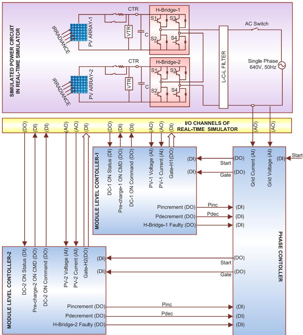
Fig. 18. Block diagram of Controller-In-Loop simulation validation of one Phase level controller card.
