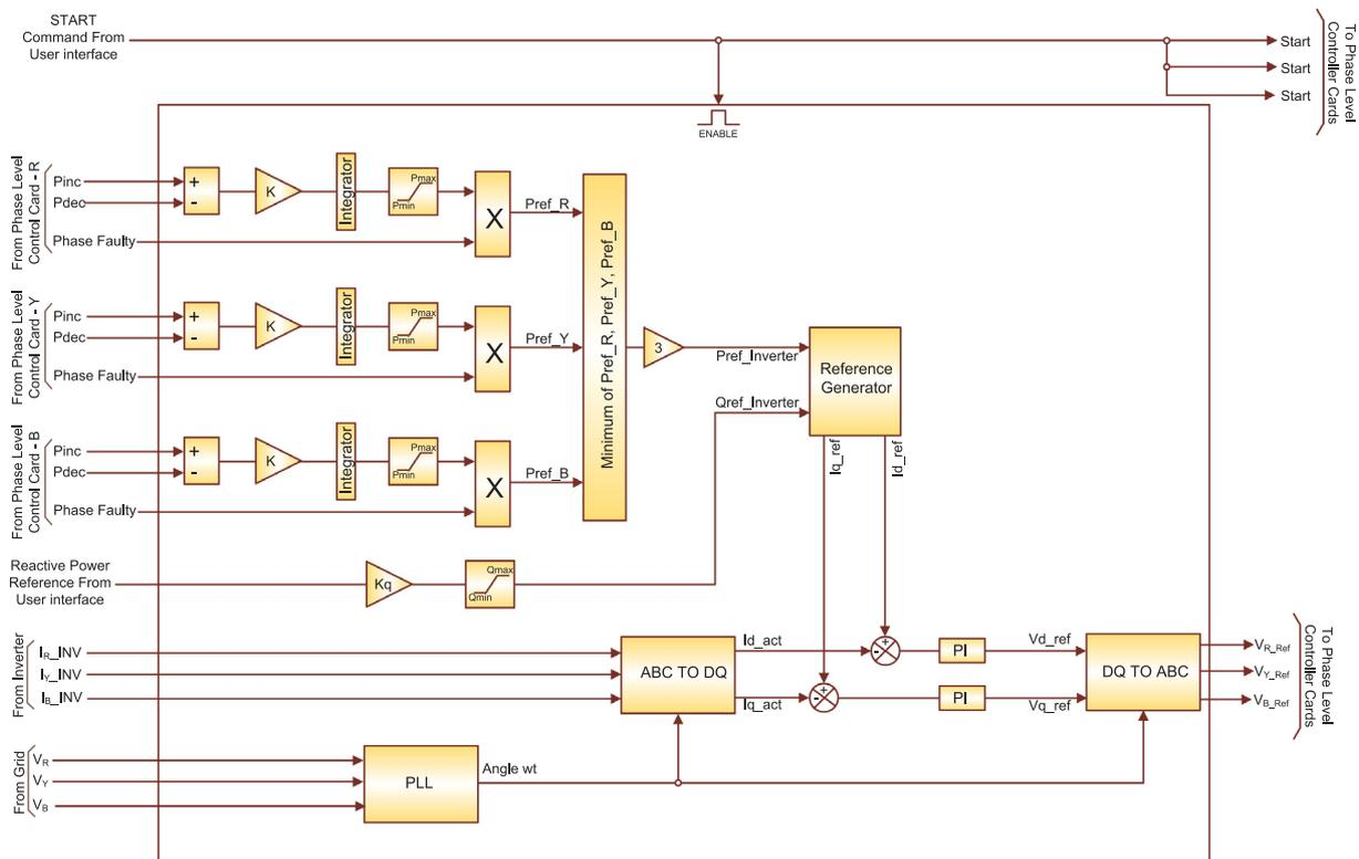
Fig. 13. A functional diagram of Master Controller Card.
