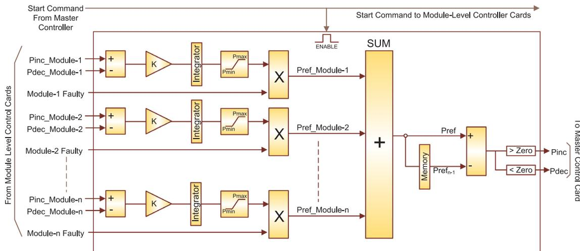
Fig. 9. The logic for reference power generation in phase level control card.
