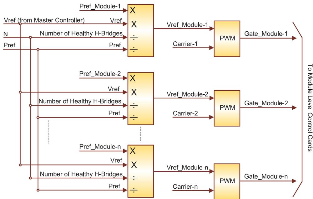
Fig. 11. The logic for Gate Pulse generation for each Module-level card.
