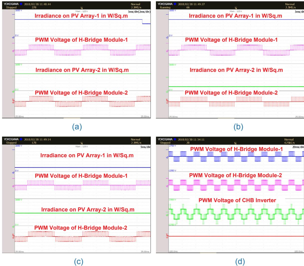
Fig. 20. (a) Output PWM voltage of each H-Bridge module when the irradiance on PV-Array-1 is equal to that of PV-Array 2. (b) Output PWM voltage of each H-Bridge module when the irradiance on PV-Array-1 is more than that of PV-Array 2. (c) Output PWM voltage of each H-Bridge module when the irradiance on PV-Array-1 is less than that of PV-Array 2. (d) PWM Voltages of each H-bridge module and the CHB Inverter PWM Voltage.
