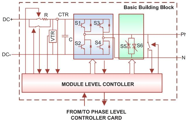
Fig. 3. Block diagram of building block for CHB inverter.
