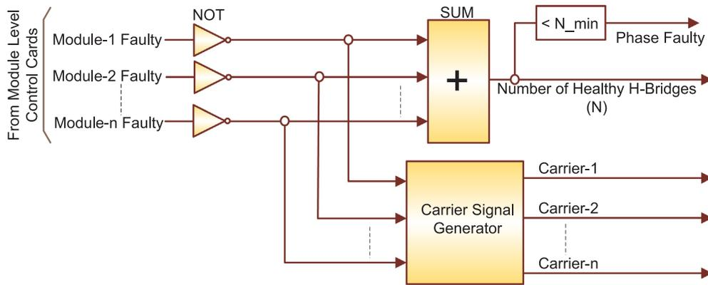
Fig. 10. The logic for generating Carrier signals and phase faulty signal in phase level control card.
