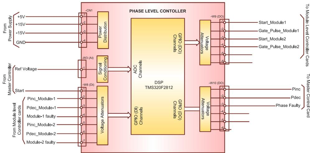
Fig. 12. Signal Exchange diagram of Phase level control card.
