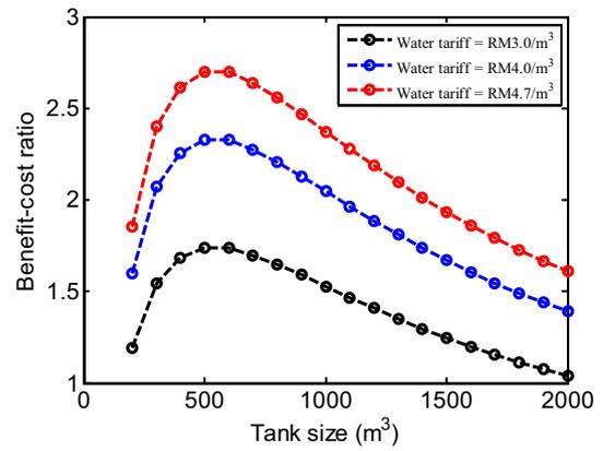
Fig. 7. Effects of tank sizes on the BCR of the proposed RWHS for the small commercial building.
