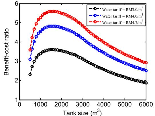
Fig. 11. Effects of tank sizes on the BCR of the proposed RWHS for the large commercial building.
