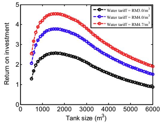
Fig. 10. Effects of tank size on the ROI for the proposed RWHS for the large commercial building.
