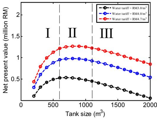
Fig. 5. Effects of tank size on the NPV of the proposed RWHS for the small commercial building.
