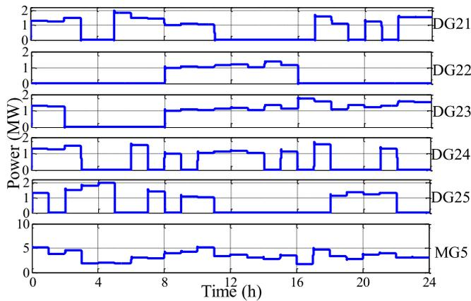
Fig. 12. DGs and MG power for MG5 at bus 13 in case of BBSA.
