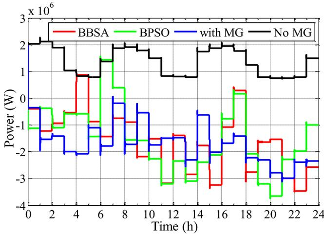
Fig. 14. Power of bus 6 compared with, without MGs and with BBSA and BPSO algorithms.
