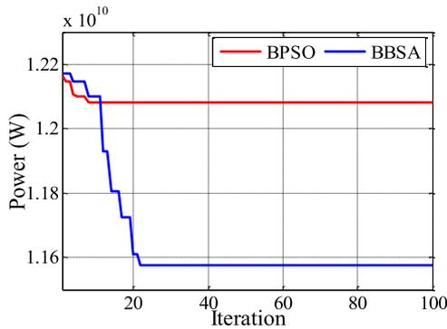
Fig. 6. BBSA and BPSO optimization of 100 iterations for the best objective function.
