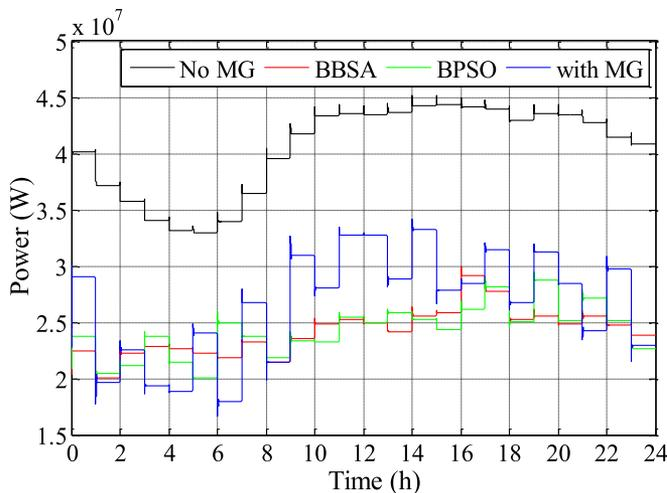
Fig. 13. Main grid power at bus 1 compared with, without MGs and with BBSA and BPSO algorithms.
