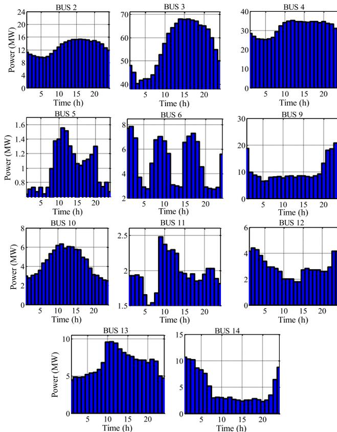
Fig. 2. Load curve for each load bus in the IEEE 14-bus test system.
