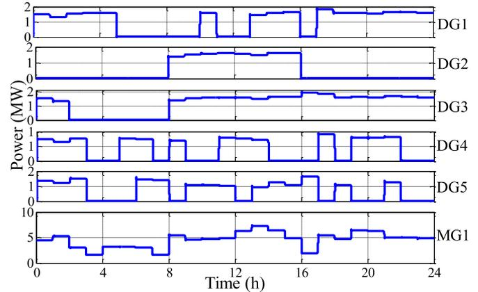
Fig. 8. DGs and MG power for MG1 at bus 5 in case of BBSA.
