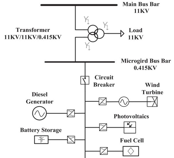
Fig. 3. Single-line diagram of the developed MG system.
