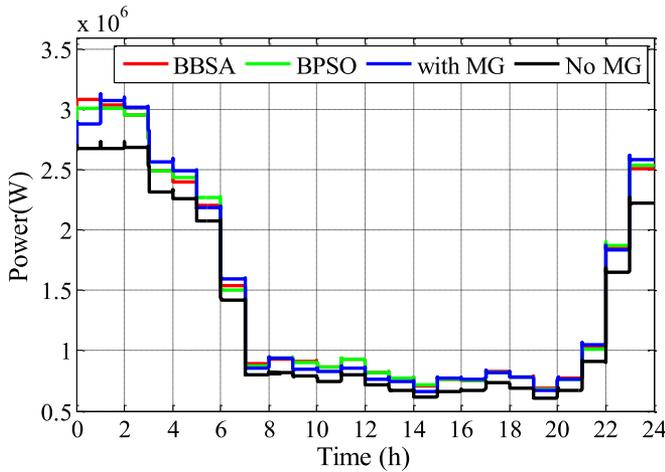
Fig. 15. Power of bus 14 compared with, without MGs and with BBSA and BPSO algorithms.
