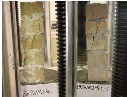
**FIGURE 7.** Failure mode of pre-wetted sediment masonry prisms
