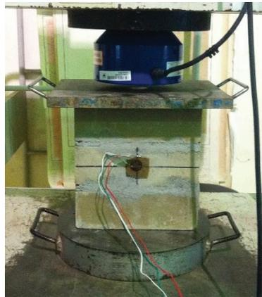
FIGURE 1. Test set-up for prism compression test
