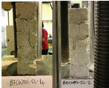
**FIGURE 8.** Failure mode of pre-wetted cement-sand masonry prisms
