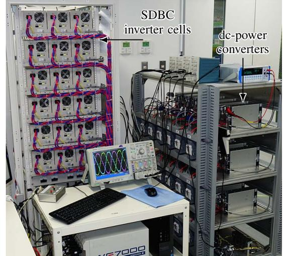
Fig. 8. Photograph of the three-phase SDBC inverter with six bridge-cells per cluster and 18 isolated dc-power converters used in experiments.
