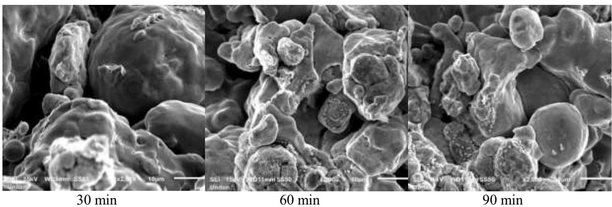
**Figure 7.** Microstructure of samples sintered at a rate of 10°C/min.
