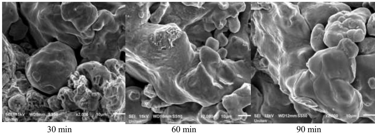
**Figure 8.** Microstructure of samples sintered at a rate of 15°C/min.
