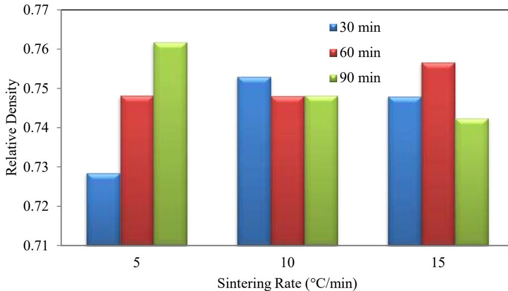
**Figure 2.** Relative density of sintered products.
