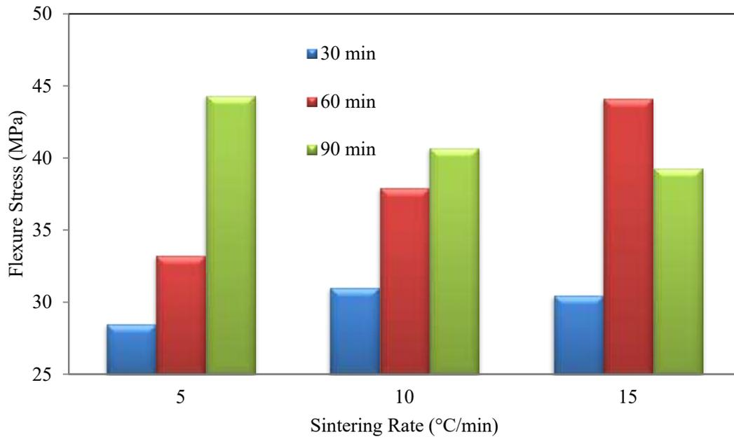
**Figure 5.** Flexure stress of sintered products.
