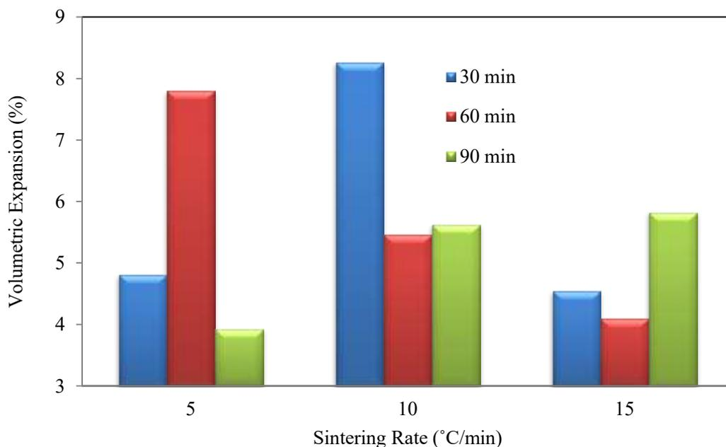
**Figure 3.** Volumetric expansion (percentage) of samples during sintering.
