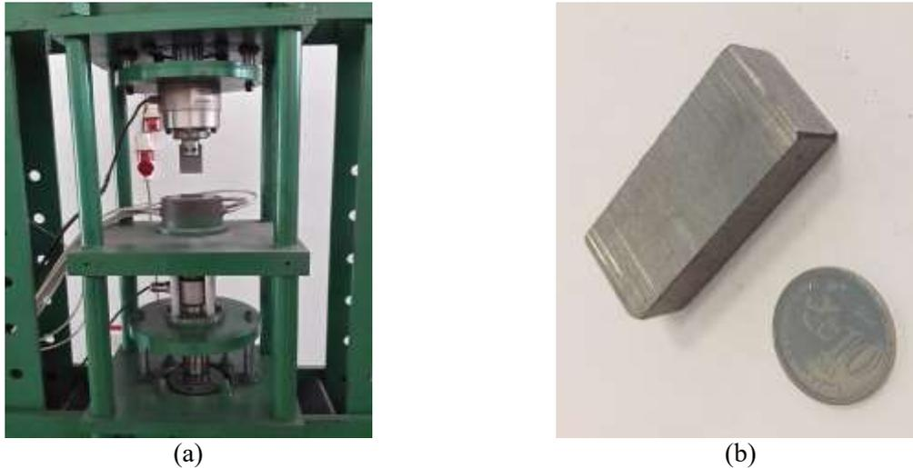
**Figure 1.** (a). T-15 compaction rig with heating system.
