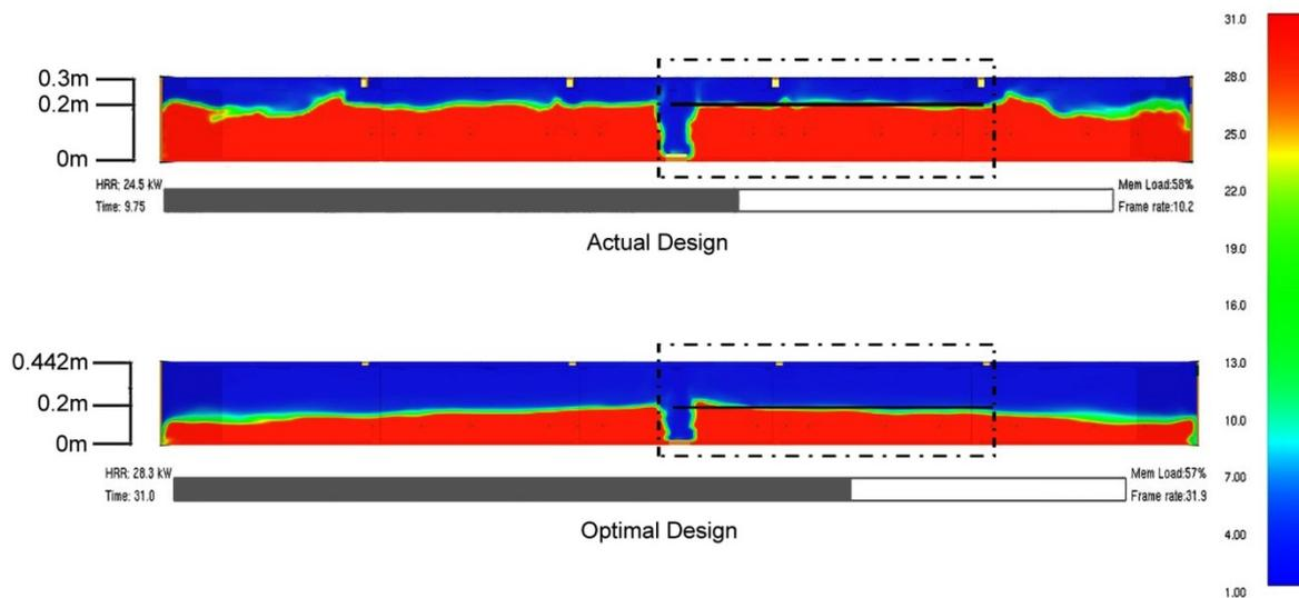
**Figure 5.** The different of smoke layer between actual and optimal design for enclosed car park.
