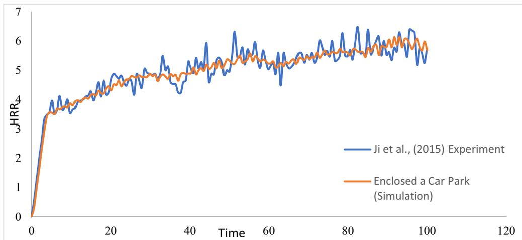
**Figure 3.** Validation between experiment and CFD simulation.
