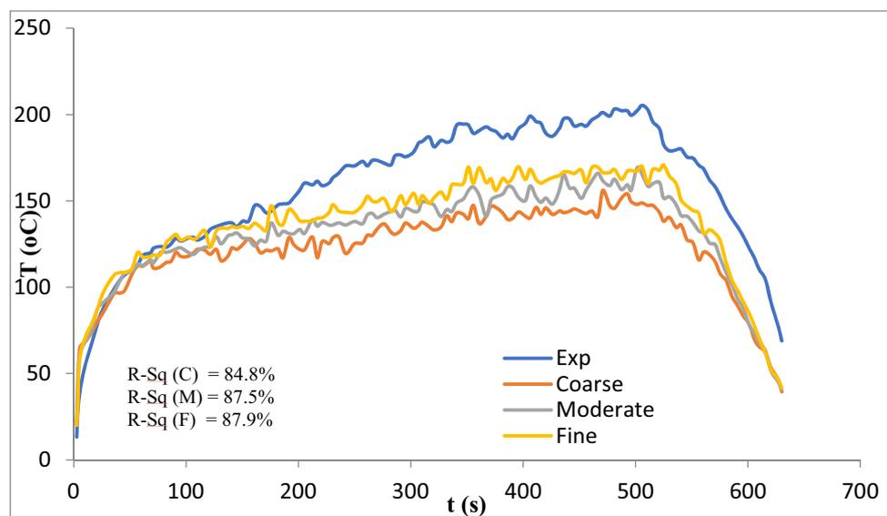
**Figure 2.** Temperatures at thermocouple tree A with 0.01 below the ceiling.
