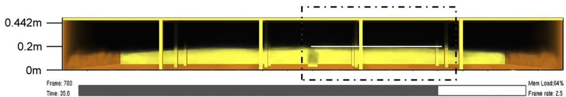
**Figure 6.** Overall smoke layer for optimal design of enclosed car park.
