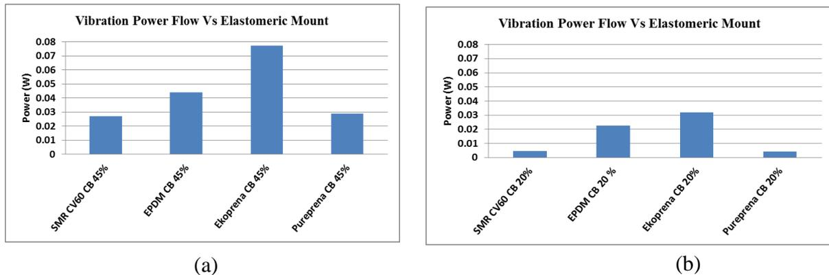
**Figure 6.** (a) Total vibration power flow through elastomeric mounts with 45% CB and (b) Total vibration power flow through elastomeric mounts with 20% CB.
