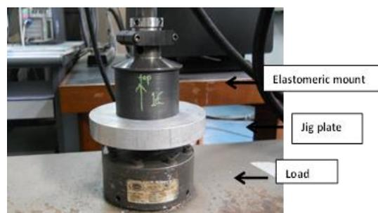
**Figure 1.** Elastomeric mount placed on a jig plate and fixed between two plates of the MTS 830 machine for static and dynamic tests.
