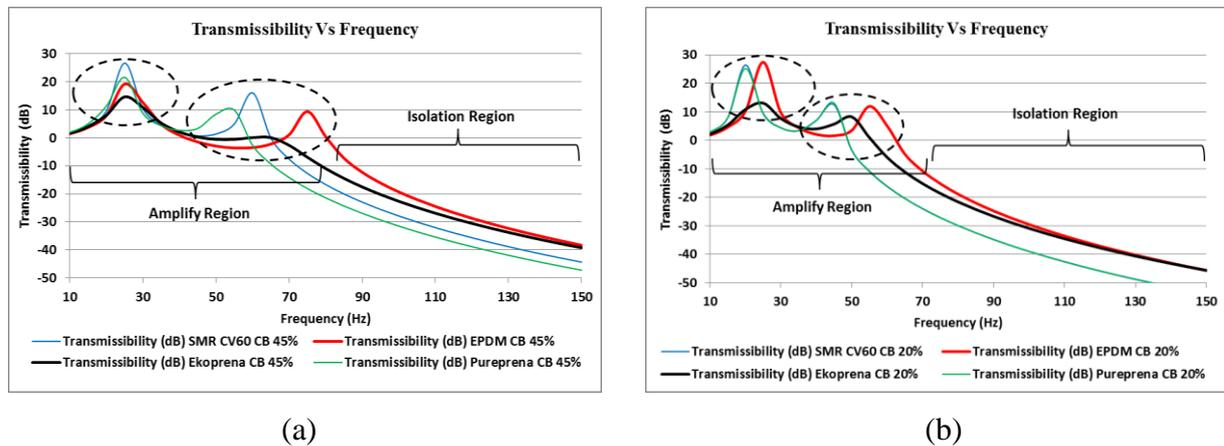
**Figure 5.** (a) Transmissibility of elastomeric mounts with 45% CB and (b) Transmissibility of elastomeric mounts with 20% CB.
