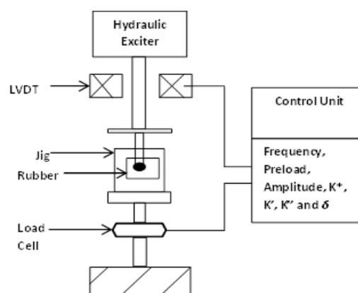
**Figure 2.** Schematic drawing of the dynamic testing machine.
