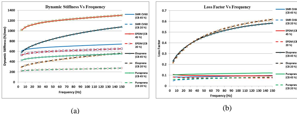
**Figure 4.** (a) Dynamic stiffness of the elastomeric mount and (b) Loss factor of the elastomeric mount.
