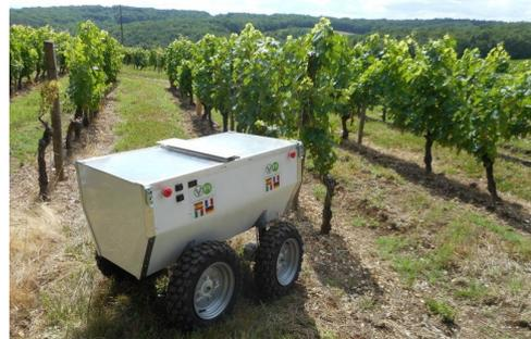
Figure 1. The VineRobot, an agriculture mobile robot, [12]
