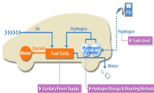
Figure 1. Mechanism of a fuel cell in vehicle [17].
