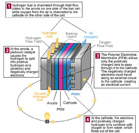
Figure 2. PEMFC Basic Operation [7].
