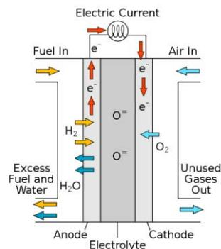
Figure 3. SOFC Basic Operation in automotive application [20].
