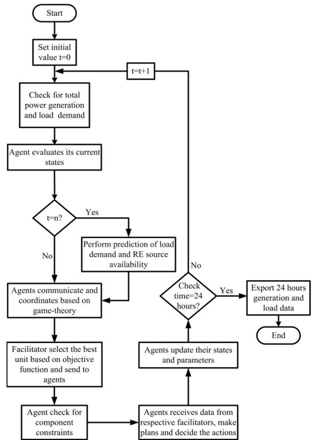
Fig. 6. MAS based EMS flowchart.
