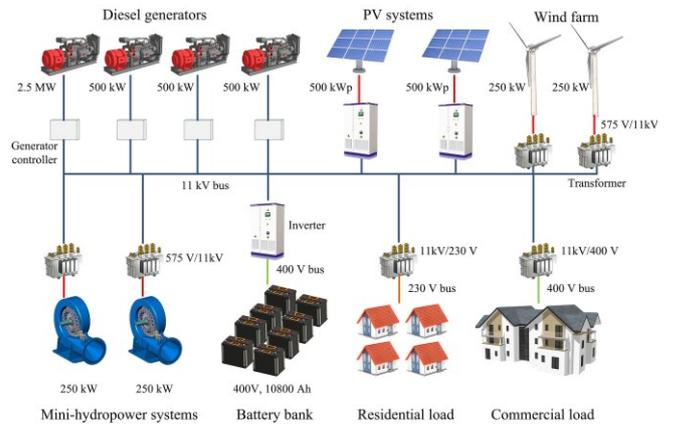
Fig. 1. Schematic of the microgrid.
