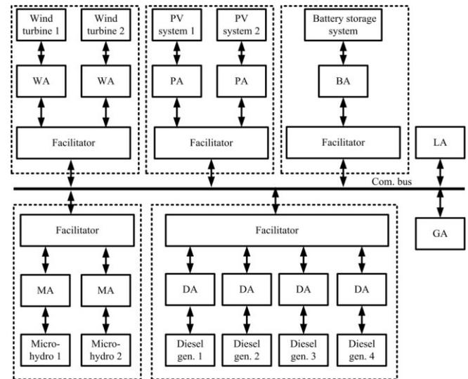
Fig. 4. MAS architecture for EMS.
