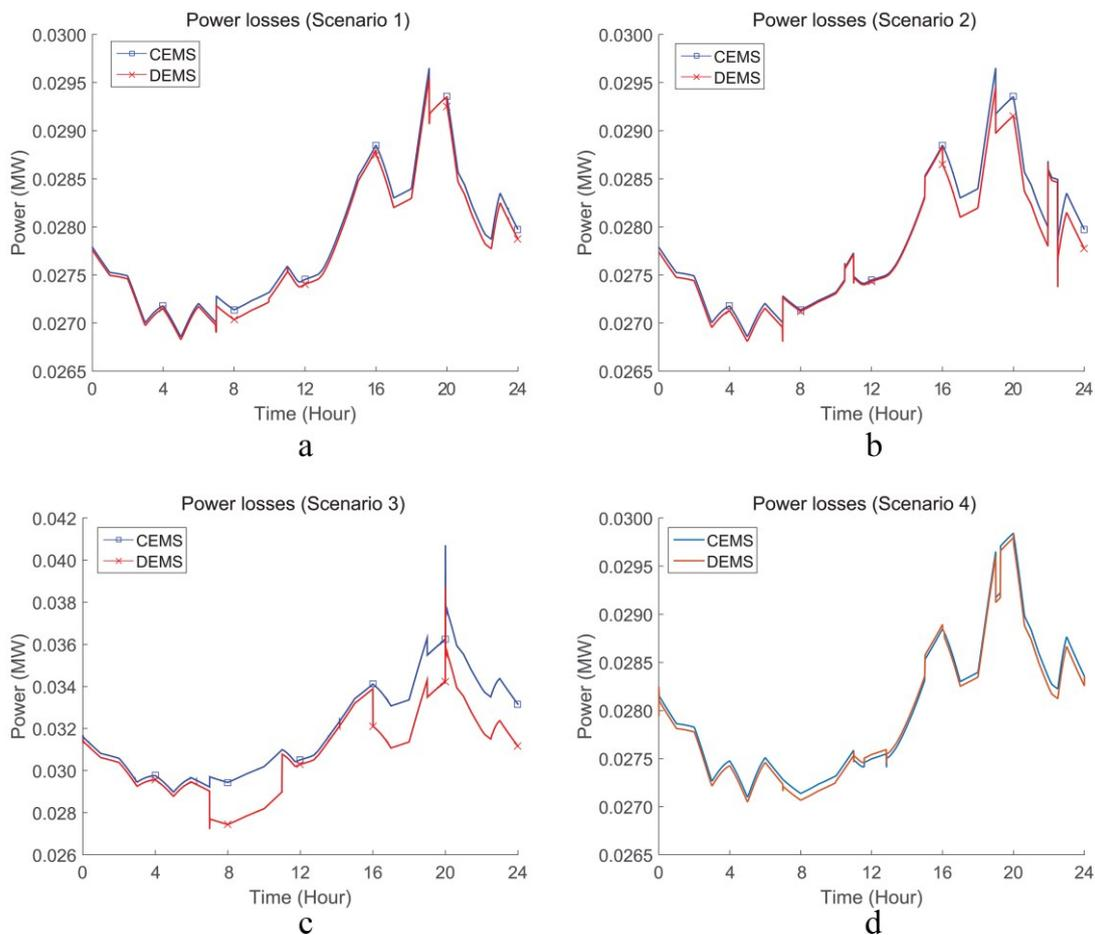
Fig. 7. Power losses for decentralized and centralized EMS a) Scenario one b) Scenario two c) Scenario three d) Scenario four.
