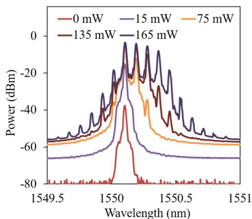
Fig. 3. Spectra of Stokes evolution as EDF pump power increases.
