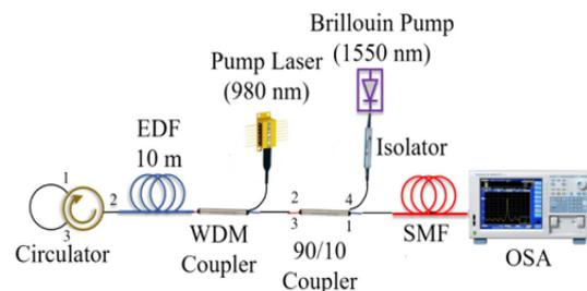
Fig. 1. Experimental setup of multiwavelength BEFL.
