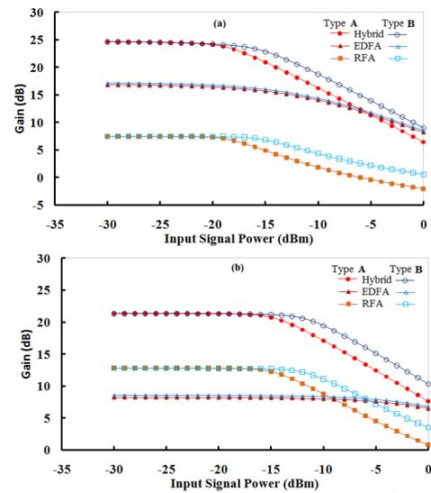
Fig. 3. Gain level vs. input signal power at two different wavelengths (a) 1560 nm and (b) 1580 nm
