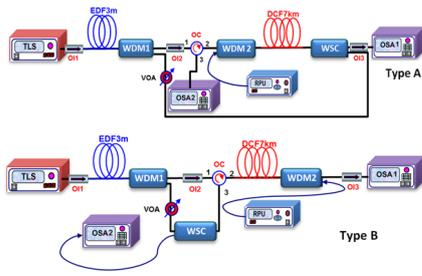
Fig. 1. Simulation setup of the serial hybrid fiber amplifier
