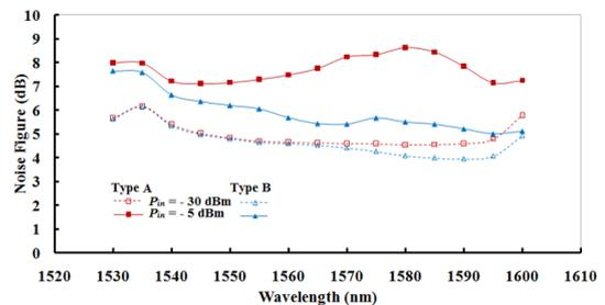
Fig. 4. Noise figure vs. wavelength for both types at the input signals of -30 dBm and -5 dBm
