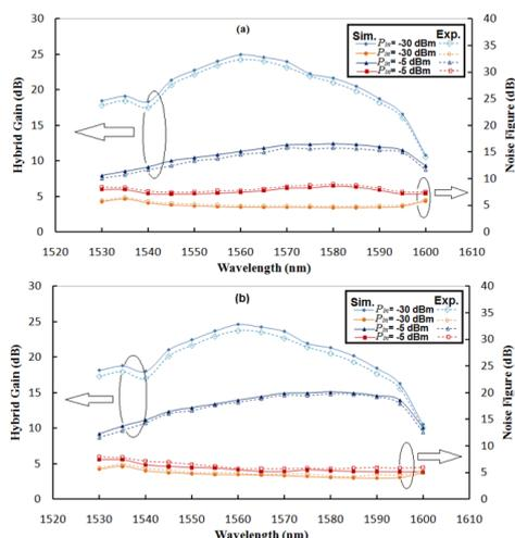
Fig. 5. Gain spectra and NF at the input signals of -30 dBm and -5 dBm for (a) Type A and (b) Type B
