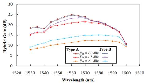
Fig. 2. Effect of the input signal power on the hybrid gain profile
