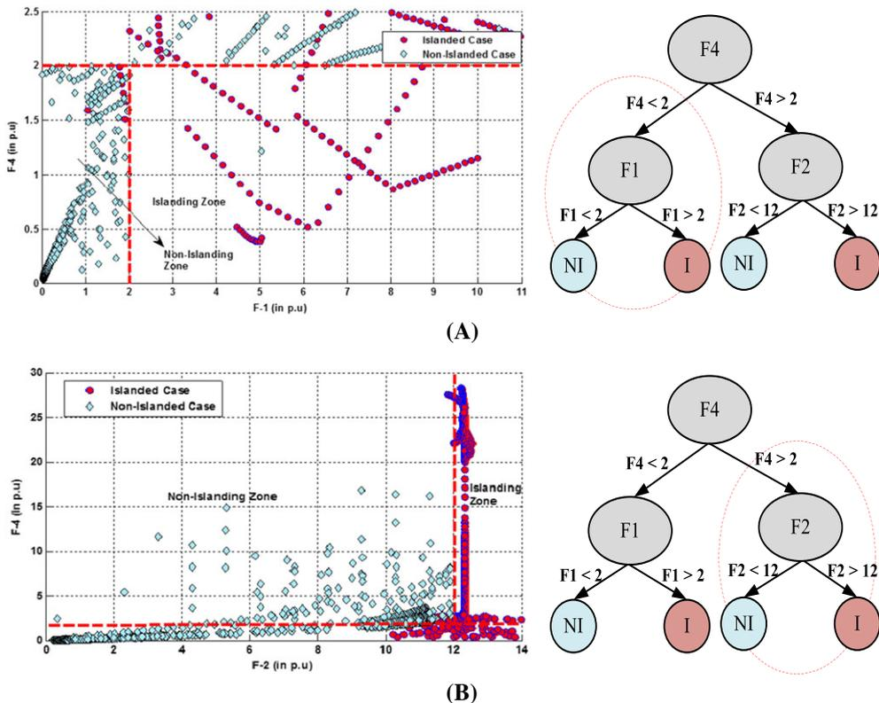
FIGURE 7 Scatter plot analysis to design a DT for setting threshold values: A, F1 versus F4 and B, F2 versus F4
