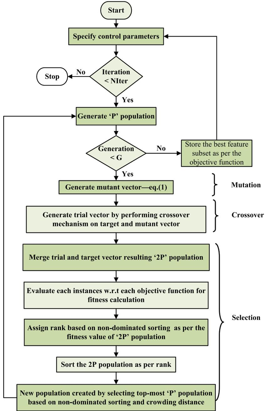
FIGURE 2 Algorithm for proposed MMODEA
