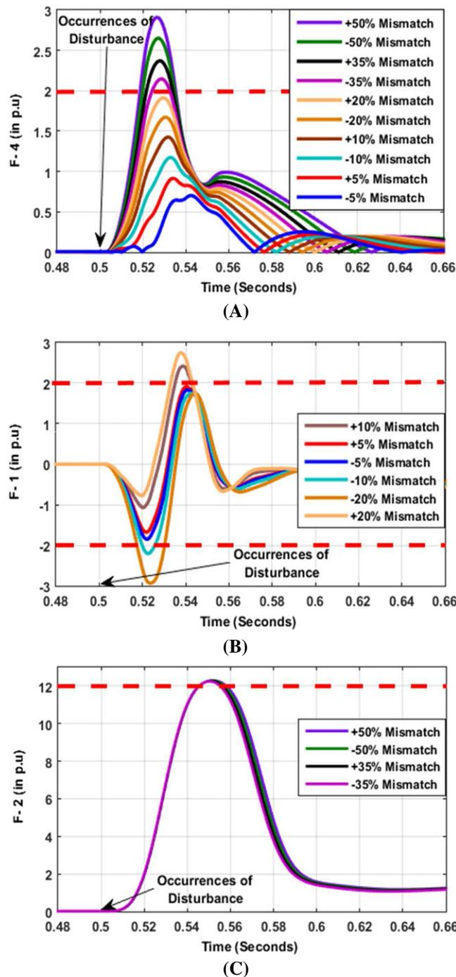
**FIGURE 10** Analysis of islanding events with reactive power load mismatch: A, variation in feature F4, B, variation in feature F1, and C, variation in feature F2
