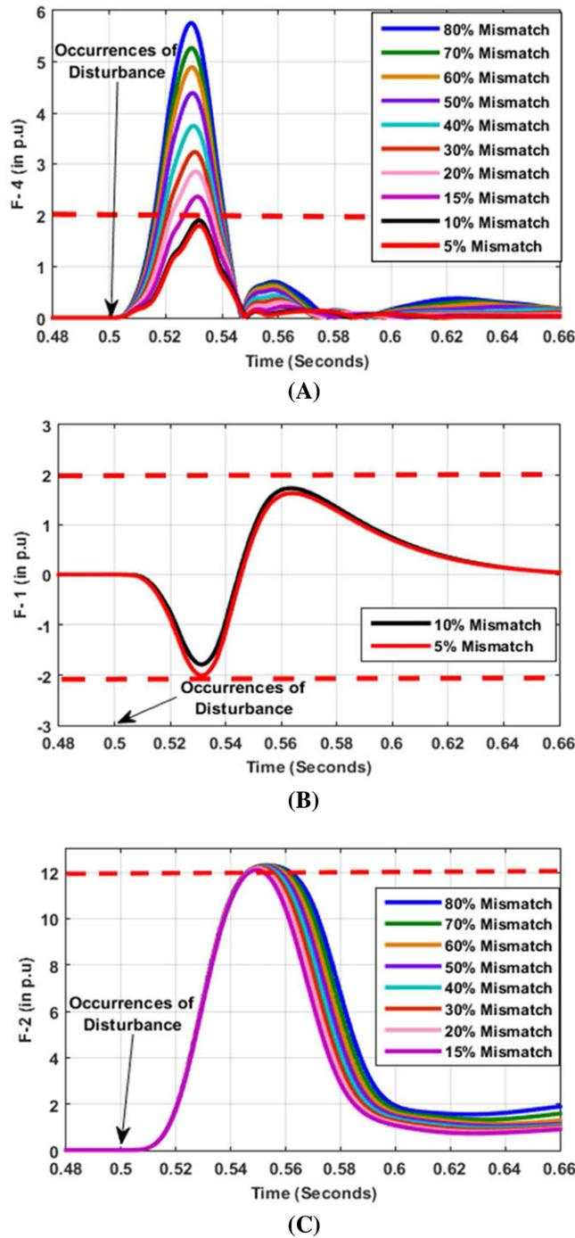
**FIGURE 9** Analysis of islanding events with active power load mismatch: A, variation in feature F4, B, variation in feature F1, and C, variation in feature F2
