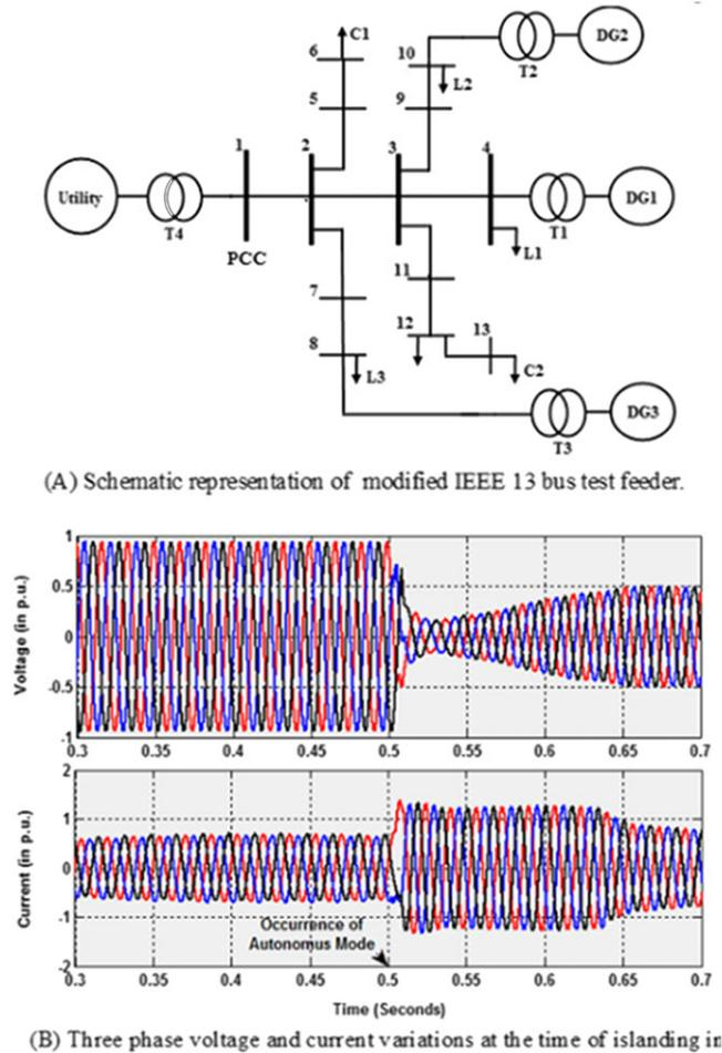
**FIGURE 1** System studied and its response. A, Schematic representation of modified IEEE 13-bus test feeder. B, Three-phase voltage and current variations at the time of islanding in DG1
