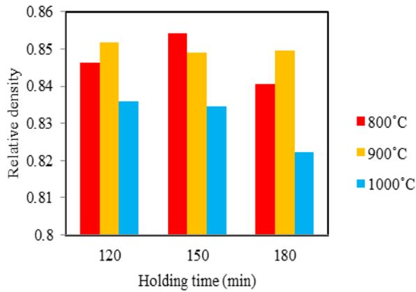
Fig. 3: Relative density of samples sintered for different holding time
