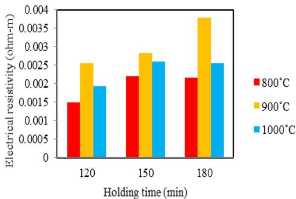
Fig. 4: Electrical resistivity of samples sintered for different holding time
