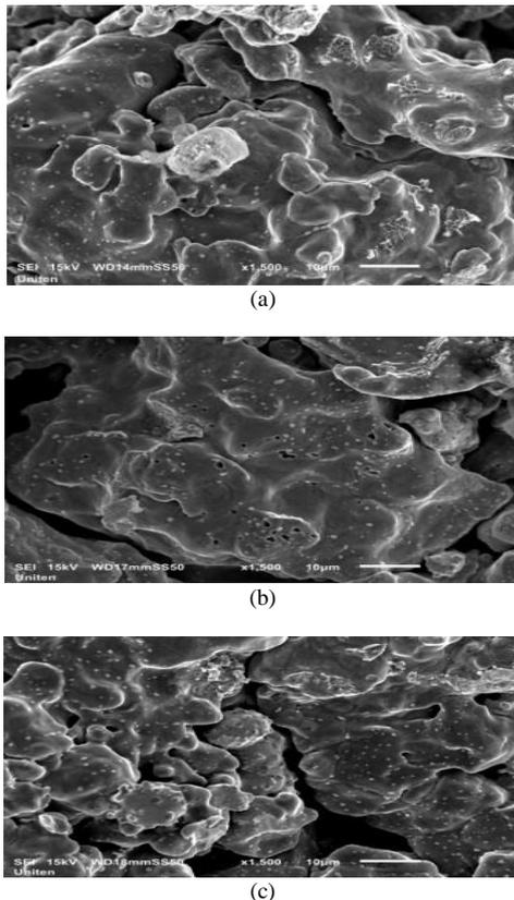
**Fig. 7:** Samples sintered at 900°C for three different holding times (a) 120 min, (b) 150 min (c) 180 min
