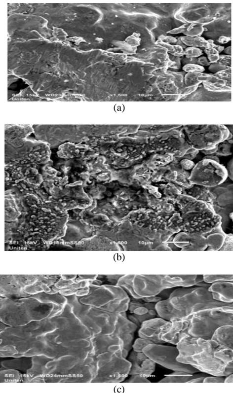
**Fig. 8:** Samples sintered at 800°C for three different holding times (a) 120 min, (b) 150 min (c) 180 min
