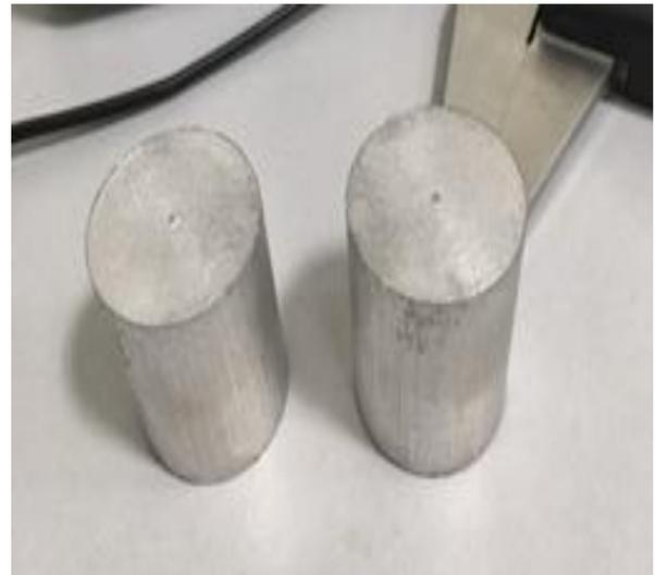
Fig. 2: Solid cylindrical shape FeCuAl green compact
