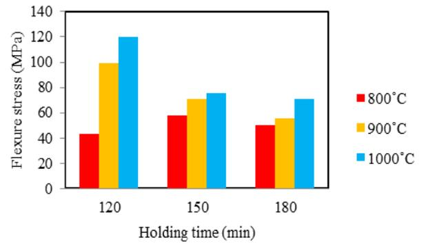
Fig. 5: Flexure stress of samples sintered for different holding time
