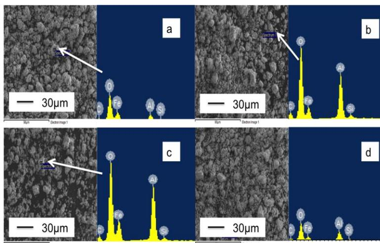
**Figure 4.** Elemental composition of  $\text{Fe}_2\text{O}_3/\text{Al}_2\text{O}_3$  when milling at different time a) 1hr b) 6hrs c) 8hrs d) 10hrs.
