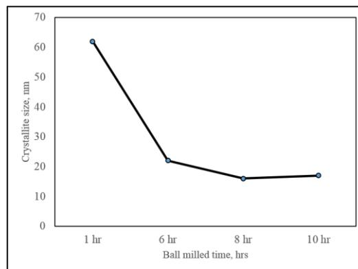
**Figure 2.** Average crystallite size of Fe<sub>2</sub>O<sub>3</sub> /Al<sub>2</sub>O<sub>3</sub> when milling at 1 hour, 6 hours, 8 hours and 10 hours.
