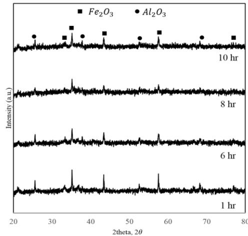
**Figure 1.** XRD result of Fe<sub>2</sub>O<sub>3</sub> /Al<sub>2</sub>O<sub>3</sub> when milling at 1 hour, 6 hours, 8 hours and 10 hours.
