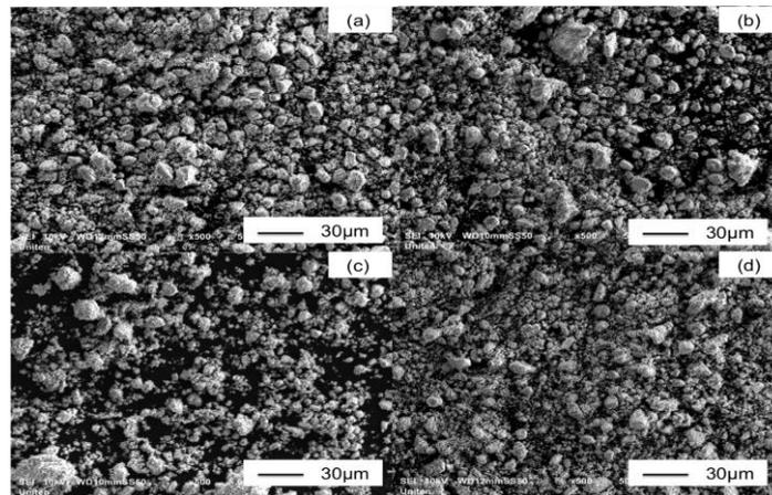
**Figure 3.** SEM images of  $\text{Fe}_2\text{O}_3/\text{Al}_2\text{O}_3$  when milling at different time a) 1hr b) 6hrs c) 8hrs d) 10hrs.
