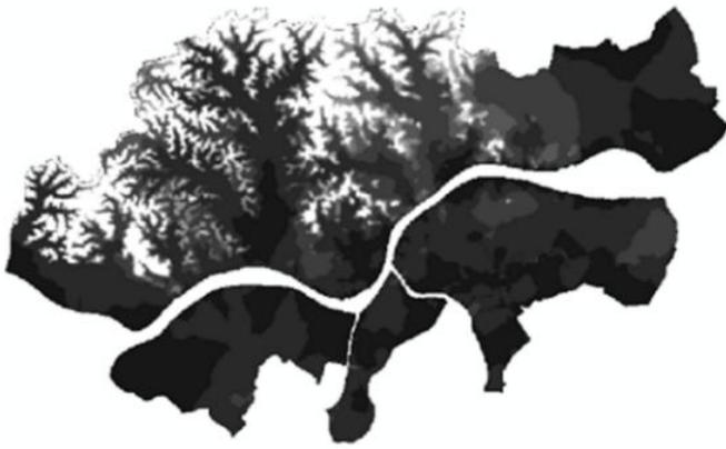
**Fig. 1:** The DEM generated based on high data using stereophotogrammetric digital technique
