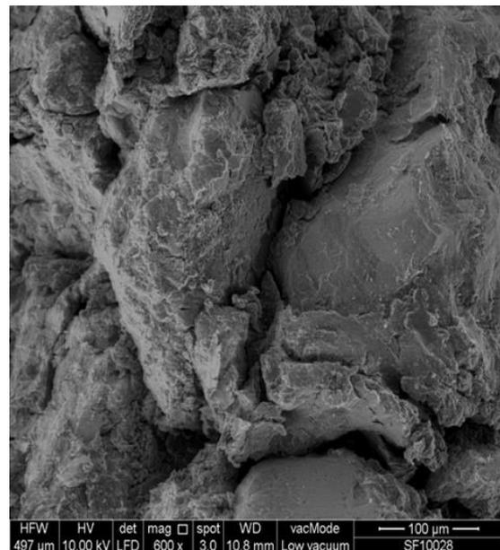
Fig 8: SEM shows bio-clogging of sand particles
