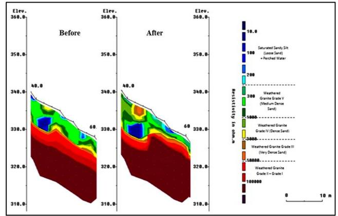
Fig. 6: Resistivity survey before and after installation of vege-grout
