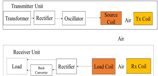
Figure 1: Transmitter and receiver unit of WPT
