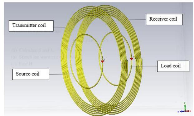
Figure 2: 4-coils system for magnetic resonance
