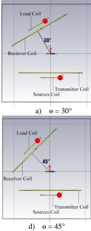
Figure 3: Rotational angle between the centre of the receiver coil and the centre point of the system,  $\theta$  of 4-coils simulation using CST microwave studio
