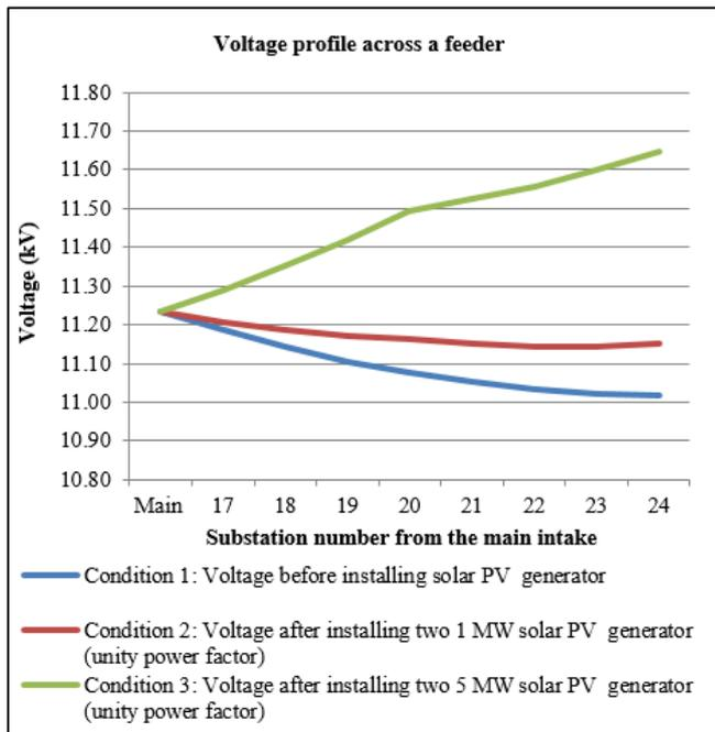
Fig. 3. Voltage Profile across the Feeders in Case 2
