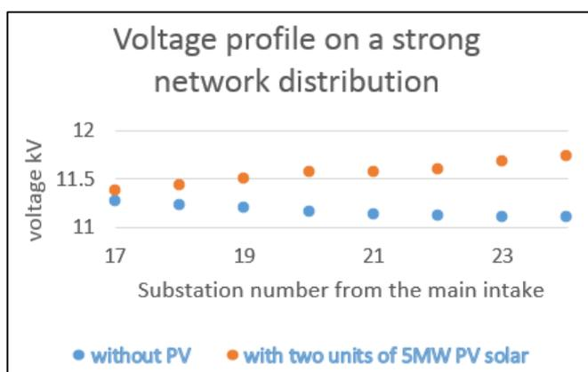
Fig. 7. Voltage Profile for Strong Network Distribution
