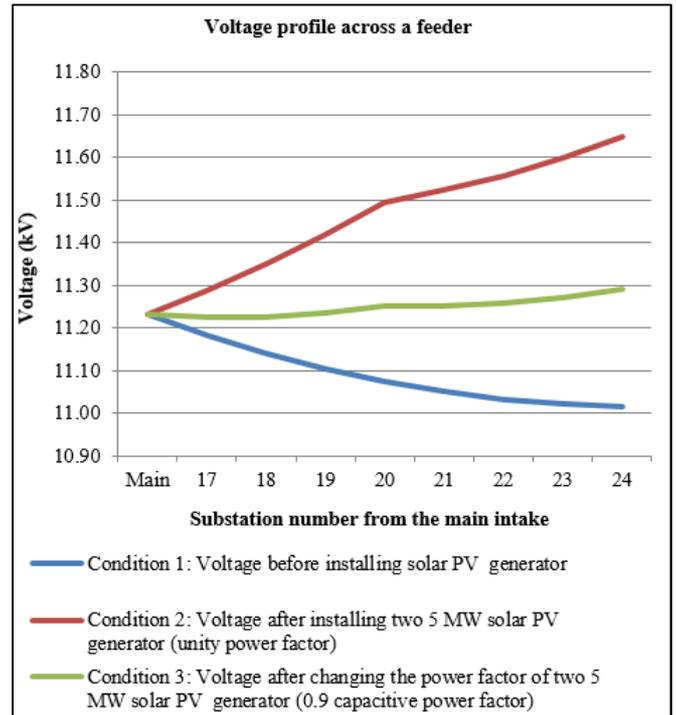
Fig. 4. Voltage Profile across the Feeders in Case 3
