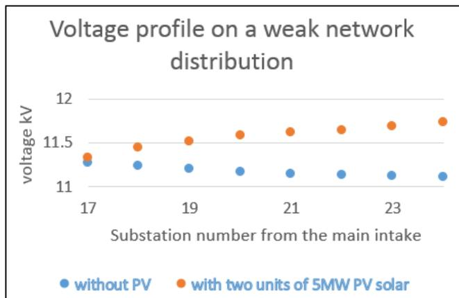
Fig. 6. Voltage Profile for Weak Network Distribution
