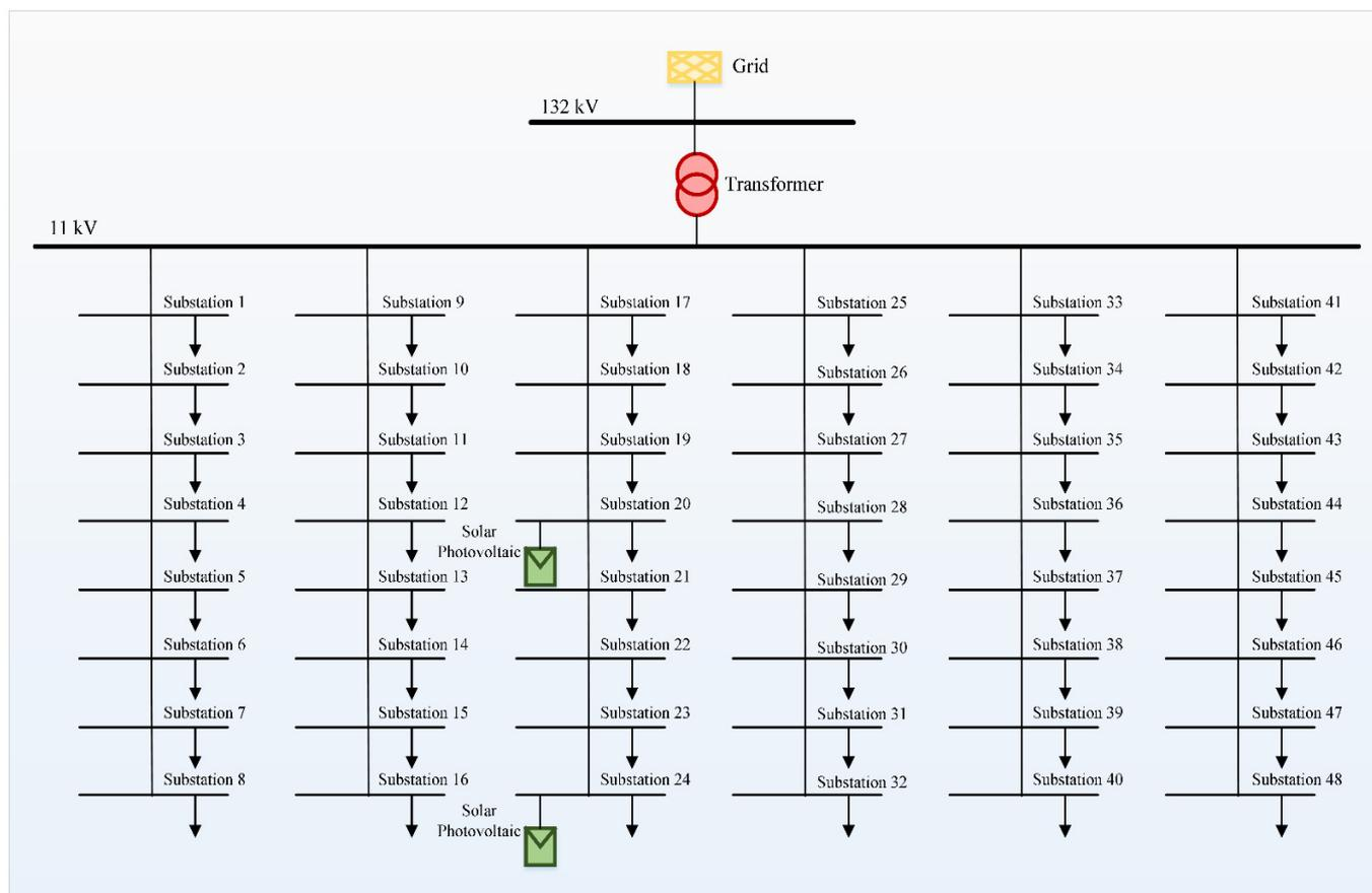
Fig. 1. A distribution network designed using DIgSILENT software
