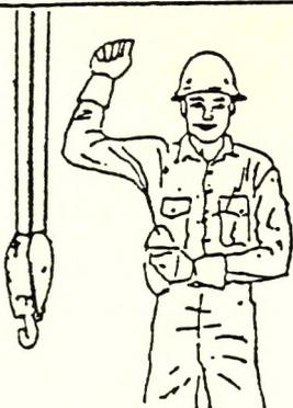
**TRAVEL.** (One Track) Lock the track on side indicated by raised fist. Travel opposite track in direction indicated by circular motion of other fist, rotated vertically in front of body. (For crawler cranes only)
