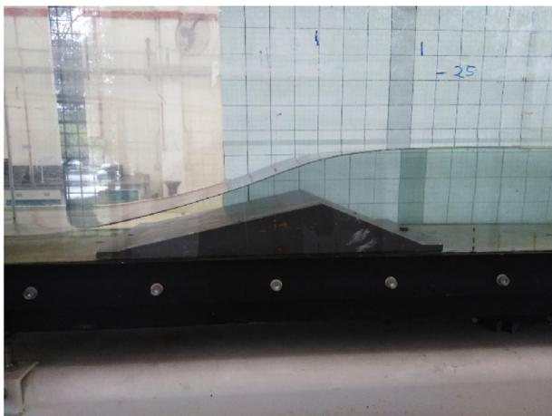
Fig. 2. Flow over hump during lab experiment.
