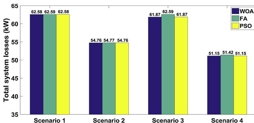
Fig. 7. Comparison of performance between WOA, FA and PSO for different scenarios with one BESS (case 1).
