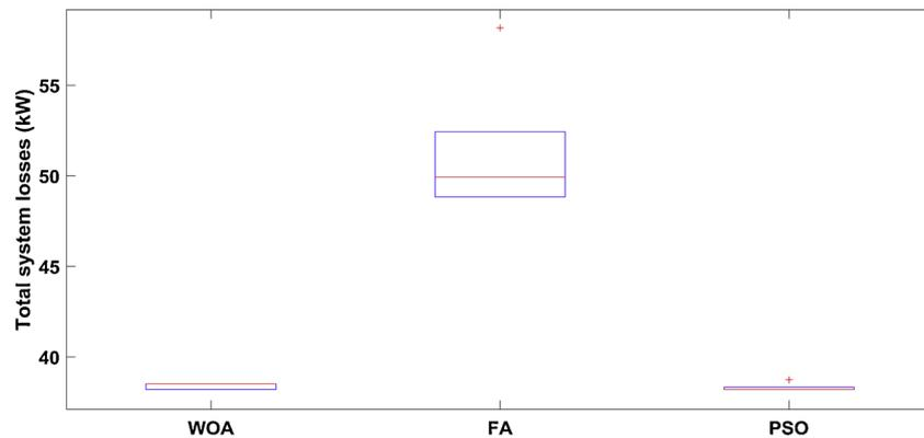
Fig. 14. Performance of WOA, FA and PSO in obtaining the optimal locations and sizing to achieve minimum total system losses (Scenario 4, case 2).
