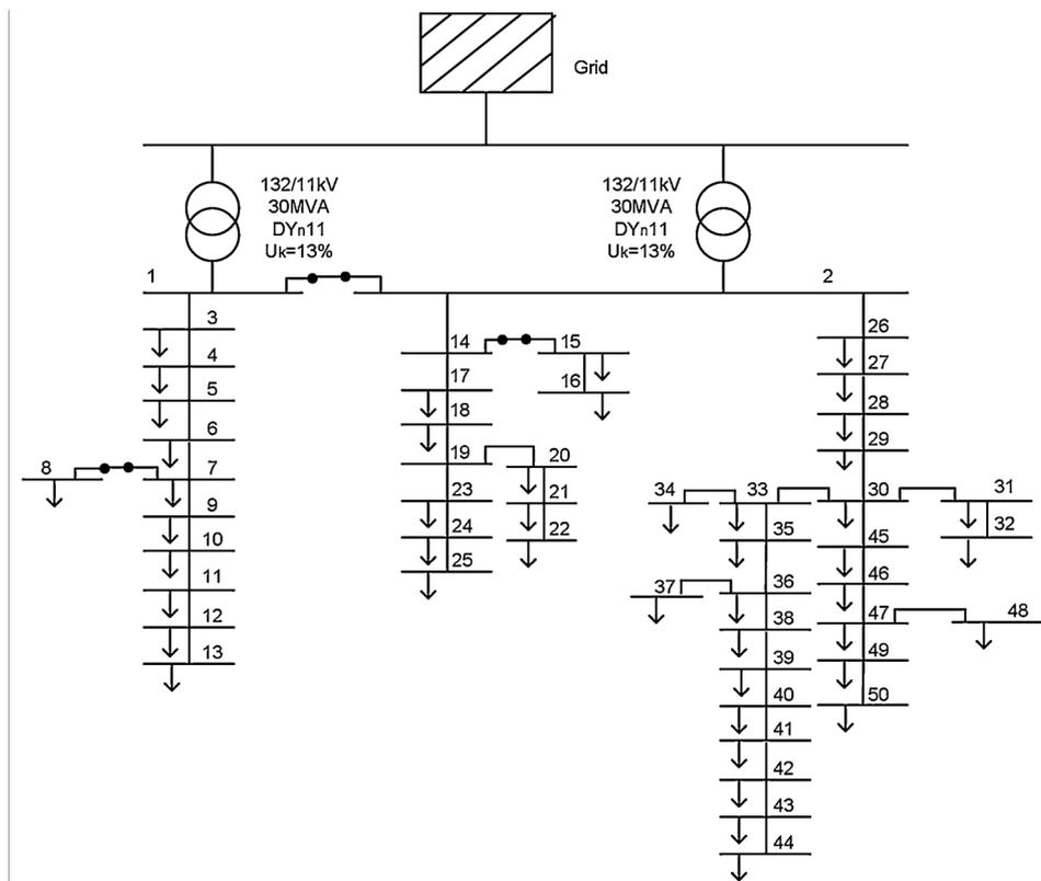
Fig. 5. Single line diagram for distribution system model.
