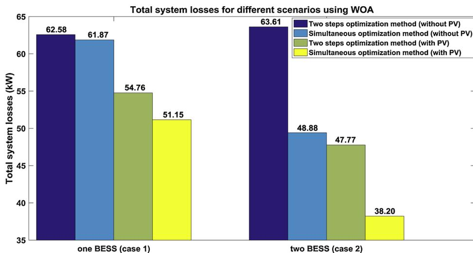
Fig. 6. Total system losses for different scenarios using WOA.
