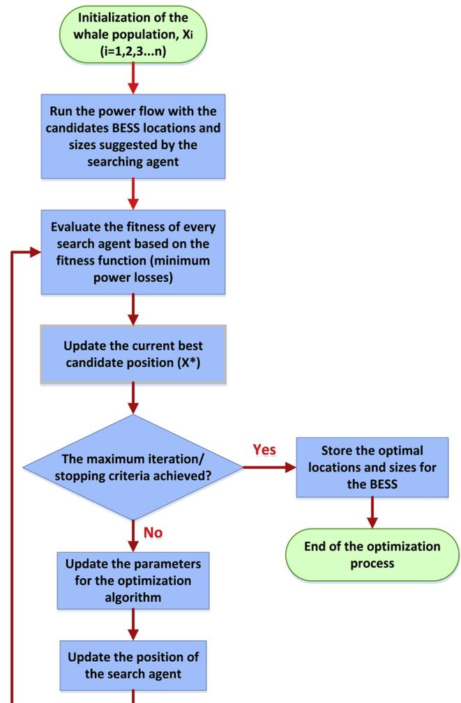
Fig. 4. The flowchart for the optimal allocation of BESS.
