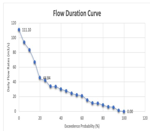
Fig. 6 Flow duration curve for Pedu Dam for 2017
