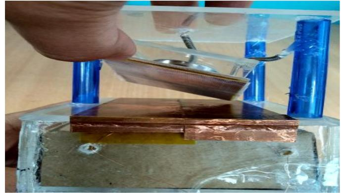
**Fig. 3 Inner side between triboelectric layers**
