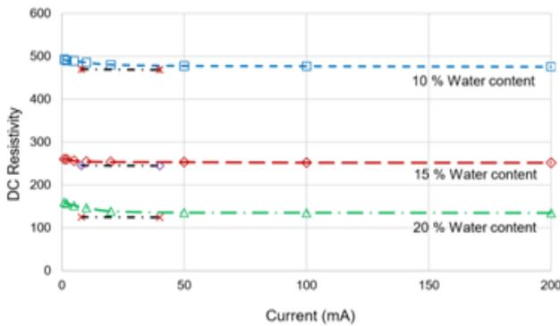
Fig. 1 Effect of water content on soil resistivity [3]
