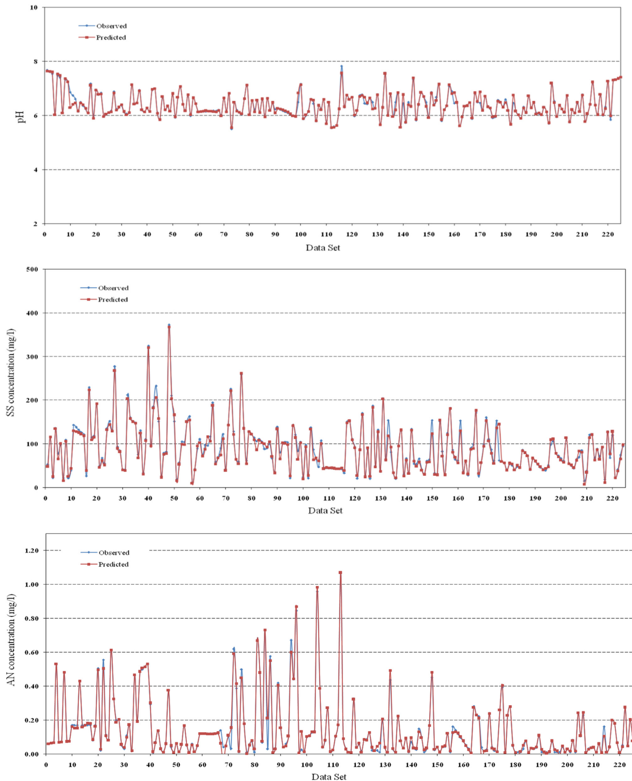
Fig. 9. Performance of the WDT-ANFIS model: A comparison between the predicted and observed values.
