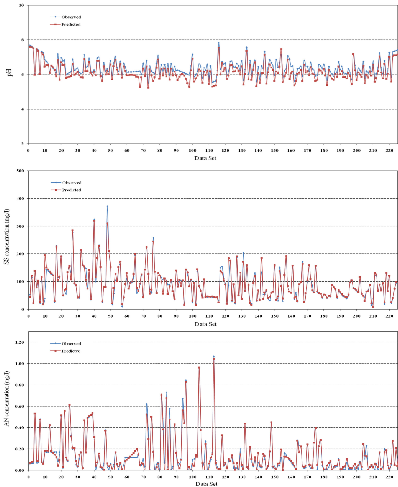
Fig. 8. Performance of the ANFIS model: A comparison between the predicted and observed values.
