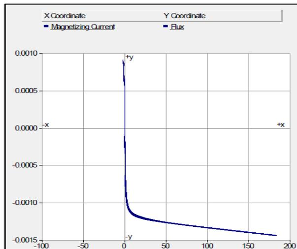
Fig. 9 Magnetization curve of WT transformer with GIC
