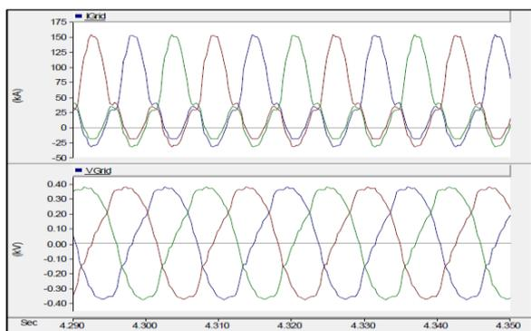
Fig. 7 Current and voltage output of Hybrid system with GIC
