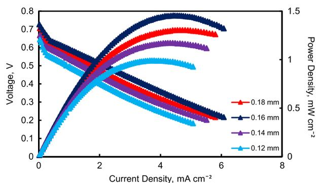
**FIGURE 3** Influence of the sodium alginate (SA) bio-membrane thickness on the passive direct methanol fuel cells (DMFCs) performance [Colour figure can be viewed at wileyonlinelibrary.com]
