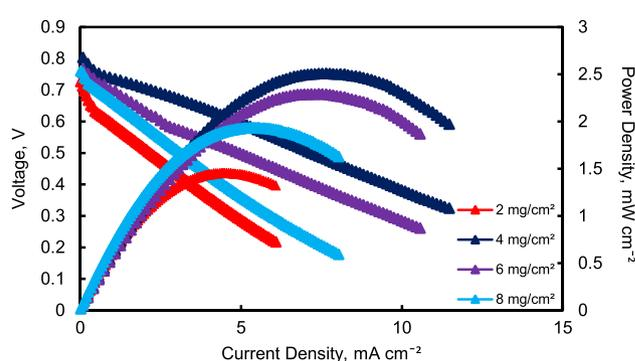
**FIGURE 4** Influence of anode catalyst loading to the sodium alginate (SA) bio-membrane on the passive direct methanol fuel cells (DMFCs) performance [Colour figure can be viewed at wileyonlinelibrary.com]
