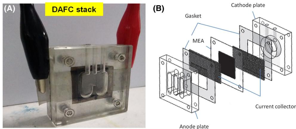
**FIGURE 2** (A) The passive direct alcohol fuel cell (DAFC) stack; (B) illustration of the DAFCs stack component [Colour figure can be viewed at [wileyonlinelibrary.com](http://wileyonlinelibrary.com)]
