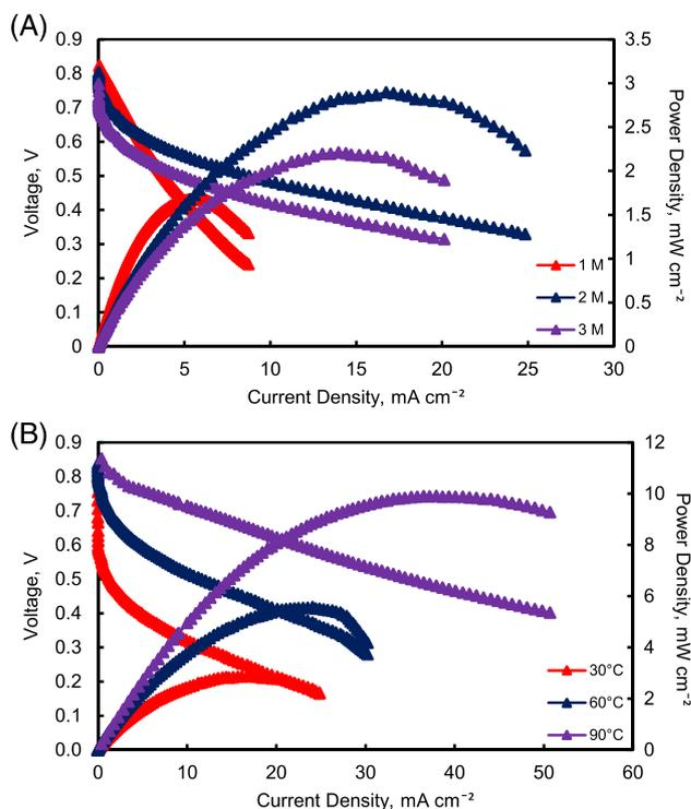
**FIGURE 7** (A) Influence of ethanol concentration and (B) influence of temperature to the sodium alginate (SA) bio-membrane on the passive direct ethanol fuel cells (DEFCs) performance [Colour figure can be viewed at wileyonlinelibrary.com]
