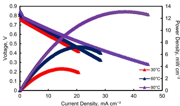
**FIGURE 6** Influence of temperature to the sodium alginate (SA) bio-membrane on the passive direct methanol fuel cells (DMFCs) performance [Colour figure can be viewed at wileyonlinelibrary.com]
