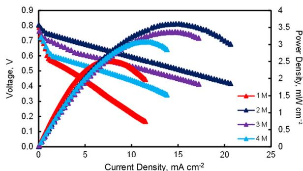
**FIGURE 5** Influence of methanol concentration to the sodium alginate (SA) bio-membrane on the passive direct methanol fuel cells (DMFCs) performance [Colour figure can be viewed at [wileyonlinelibrary.com](http://wileyonlinelibrary.com)]
