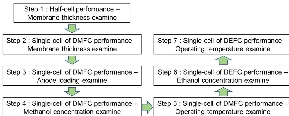
**FIGURE 1** The experimental works for the self-synthesis sodium alginate (SA) bio-membrane. DEFC, direct ethanol fuel cell; DMFC, direct methanol fuel cell [Colour figure can be viewed at [wileyonlinelibrary.com](http://wileyonlinelibrary.com)]
