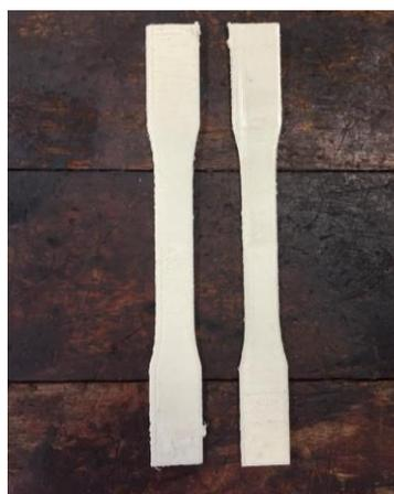
Fig. 4 Tensile specimen fabricated via 3D printing machine following ASTM D638 standard.
