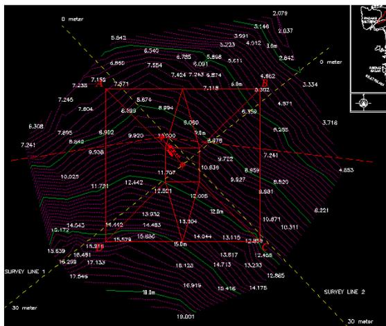
Fig. 1 Resistivity Survey Lines at T22 TelukApau, Langkawi Island
