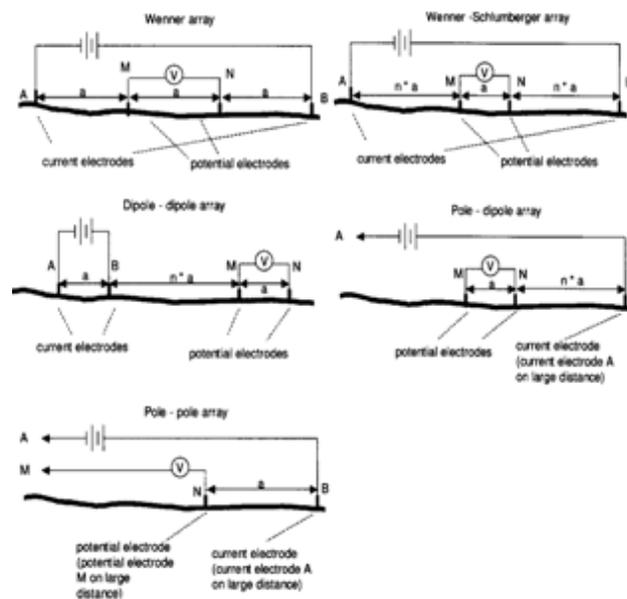
Fig. 3 Various arrays for current and potential electrodes
