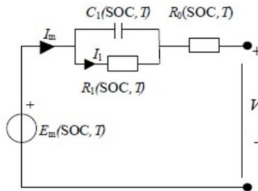
Fig. 2. Single RC block model of lithium ion battery cell
