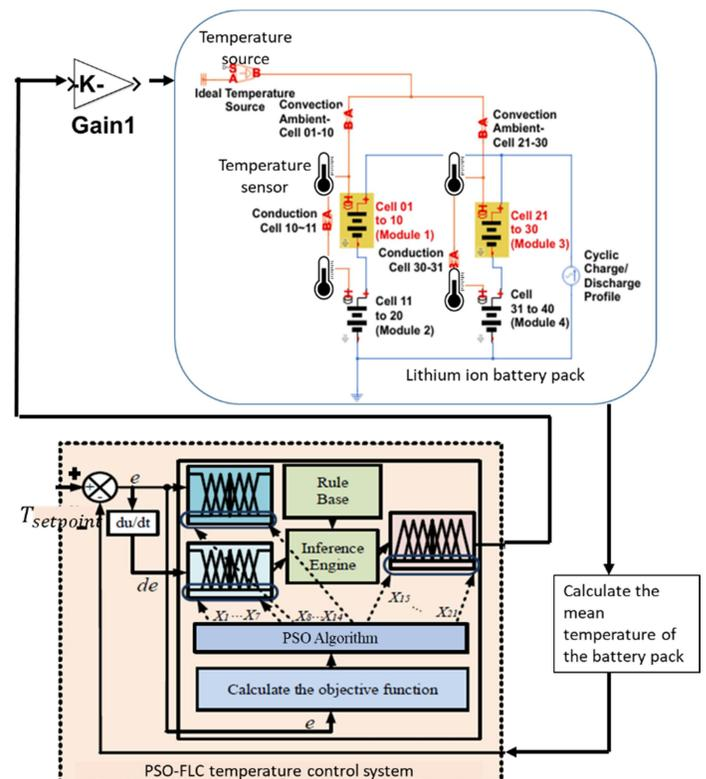
Fig. 1. Lithium ion battery pack thermal management system using PSO based fuzzy algorithm
