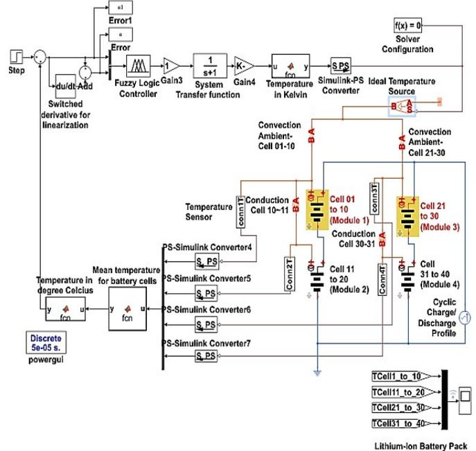
Fig. 7. Simulation model for battery temperature control system
