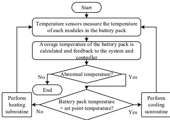
Fig. 8. Temperature regulation scheme of the lithium ion battery pack
