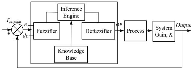
Fig. 4. Structure of Fuzzy based control system
