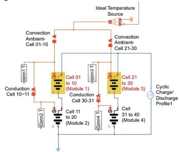
Fig. 3. Lithium ion battery pack configuration with temperature source
