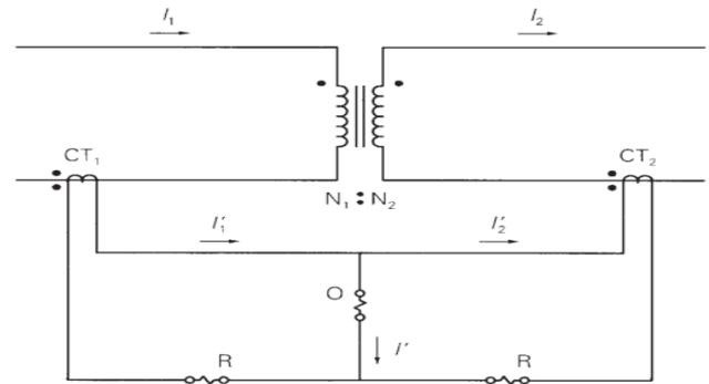
Fig. 2. Differential protection for a 2-winding power transformer.
