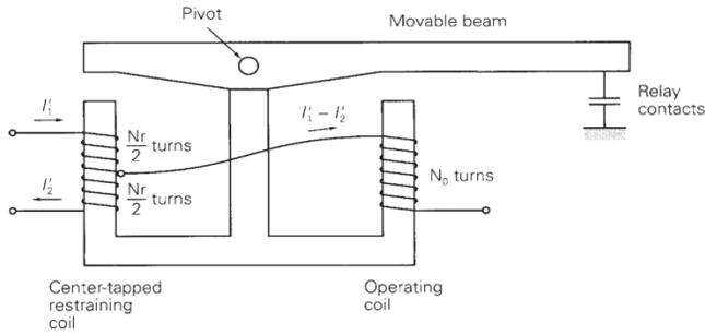
Fig. 3. Balance beam differential protection relay structure.
