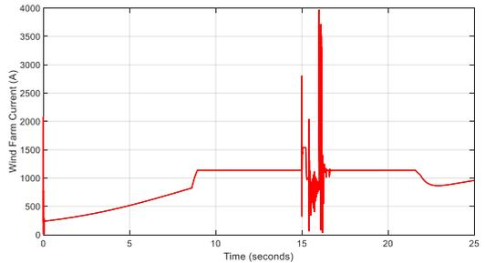
Fig. 19. Aggregated wind farm current flow during external three phase fault at the grid.
