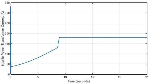
Fig. 7. Intertie power transformer current flow during normal operation.
