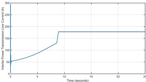
Fig. 8. Intertie power transmission line current flow during normal operation.
