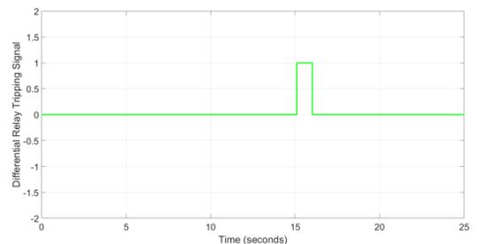
Fig. 12. Transformer differential relay successful operation during internal fault at the intertie power transformer.
