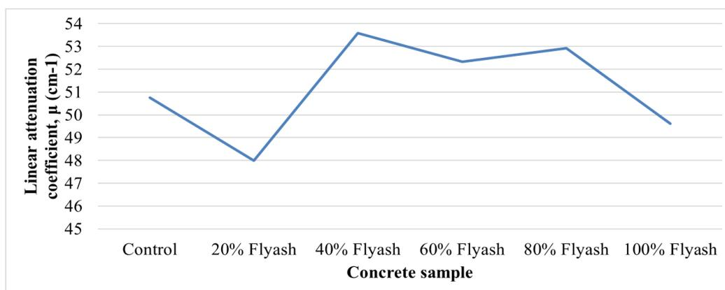
**Figure 4.** Linear attenuation coefficient for each concrete samples.
