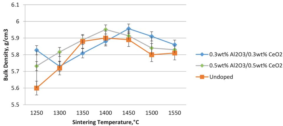
Figure 1. Effect of CeO<sub>2</sub> and Al<sub>2</sub>O<sub>3</sub> additions on the bulk density of 3Y-TZP sintered between 1250–1550°C.
