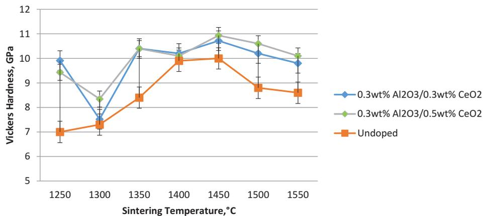
Figure 2. Effect of CeO<sub>2</sub> and Al<sub>2</sub>O<sub>3</sub> additions on the Vickers hardness of 3Y-TZP sintered from 1250°C to 1550°C.
