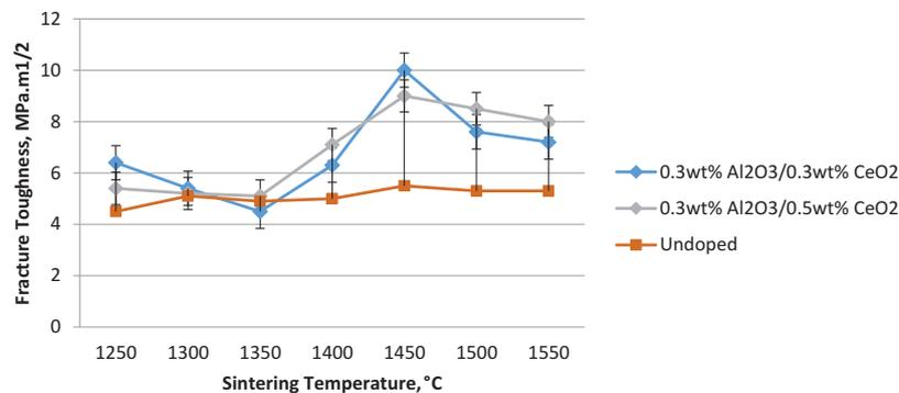
Figure 3. Influence of dopant additions and sintering temperature on the fracture toughness of 3Y-TZP.
