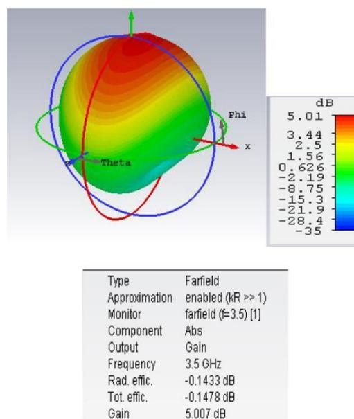
**Figure 4.** Farfield Radiation Pattern in 3D Form
