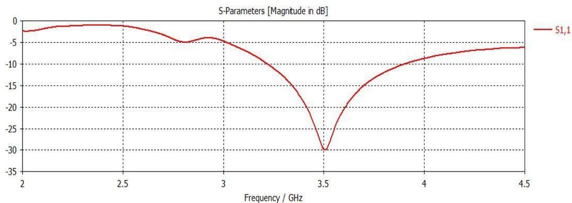
**Figure 3.** Return Loss or S11 Parameter of the Designed Antenna
