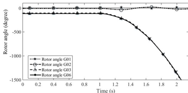
Figure 1. Instability occurrence in IEEE 14-Bus test system.
