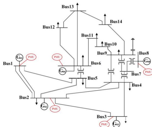
Figure 4. Single line diagram of IEEE 14-bus test system and PMU locations.
