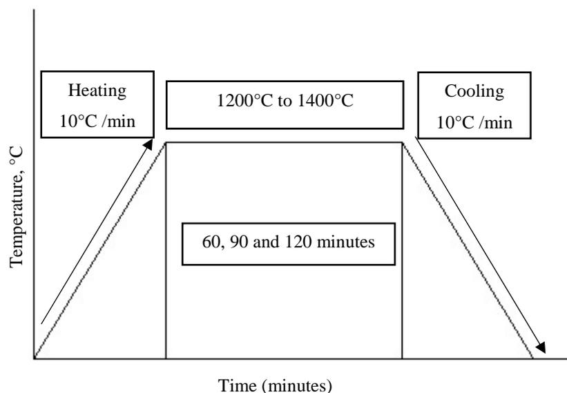
**Figure 1: Graph of Sintering profile**
