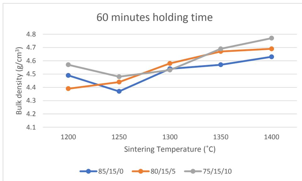
Figure 2: The effect of Bulk density on sintering temperature for 60 minutes holding time
