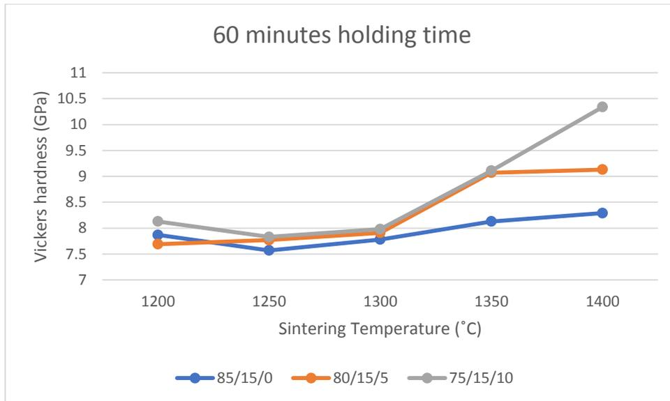
**Figure 5: The effect of Vickers hardness on sintering temperature for 60 minutes holding time**
