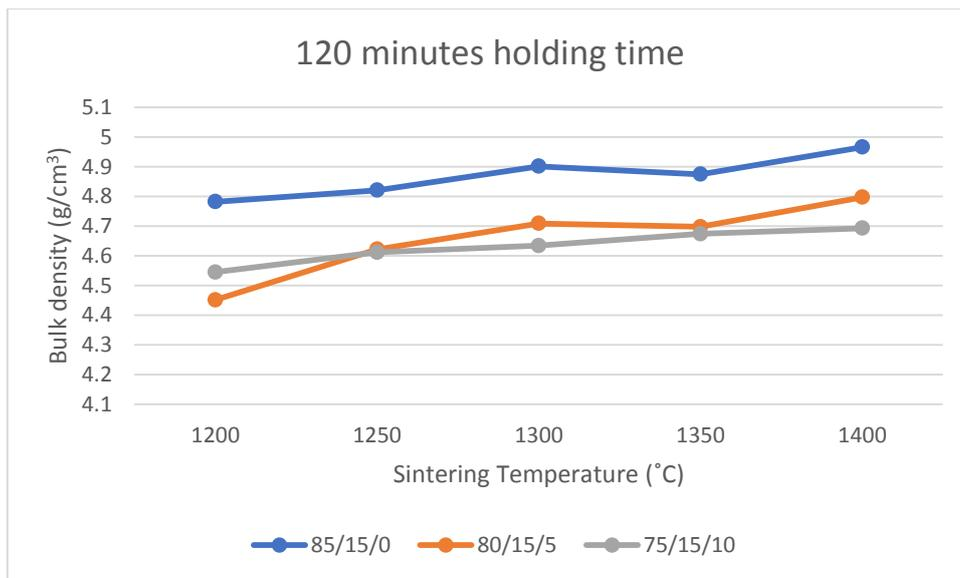
**Figure 4: The effect of Bulk density on sintering temperature for 120 minutes holding time**
