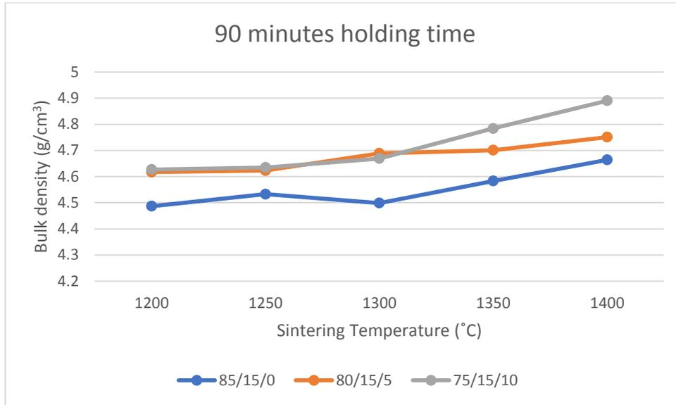
**Figure 3: The effect of Bulk density on sintering temperature for 90 minutes holding time**
