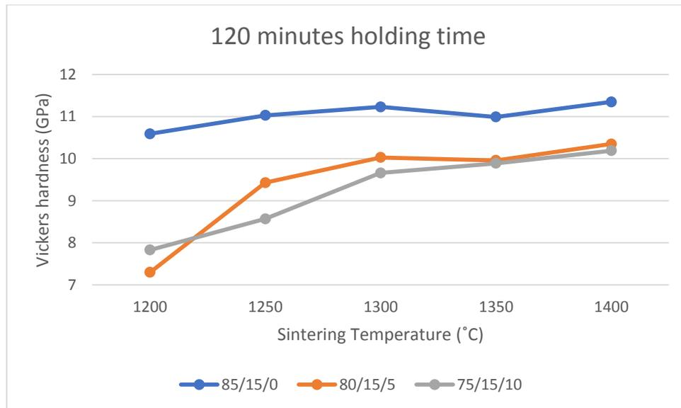
Figure 7: The effect of Vickers hardness on sintering temperature for 120 minutes holding time
