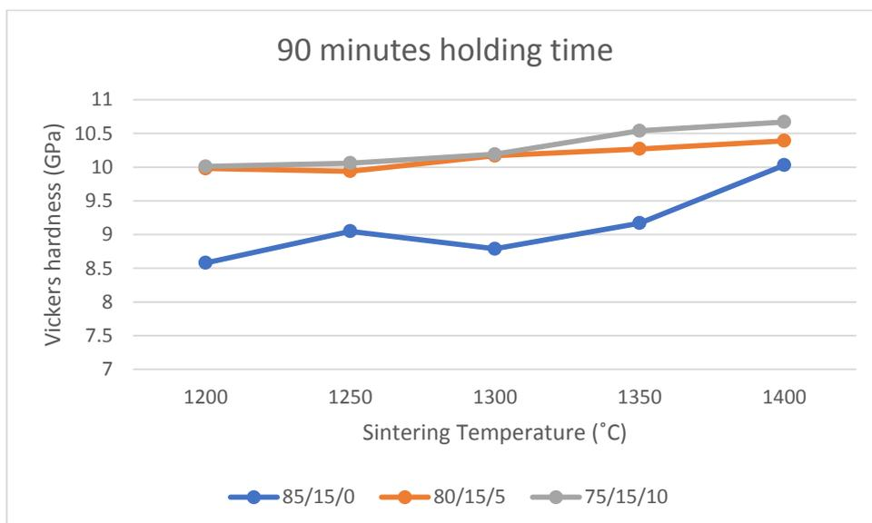
**Figure 6: The effect of Vickers hardness on sintering temperature for 90 minutes holding time**
