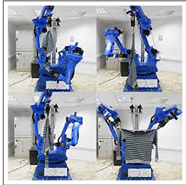
Figure 5. Robot unfolding a shirt.<sup>69</sup>
