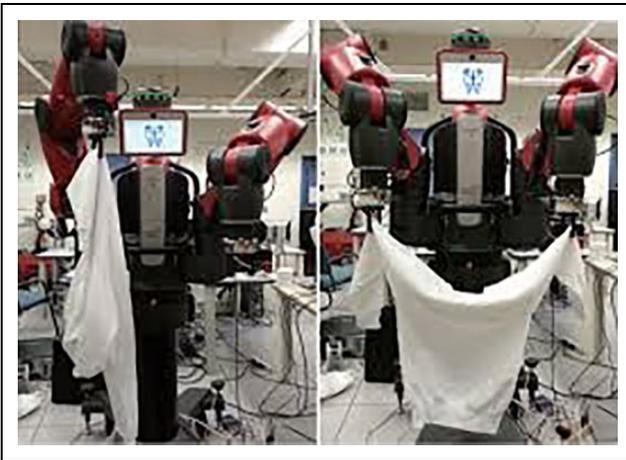
Figure 7. Baxter recognize the pose and unfold a garment.<sup>76</sup>
