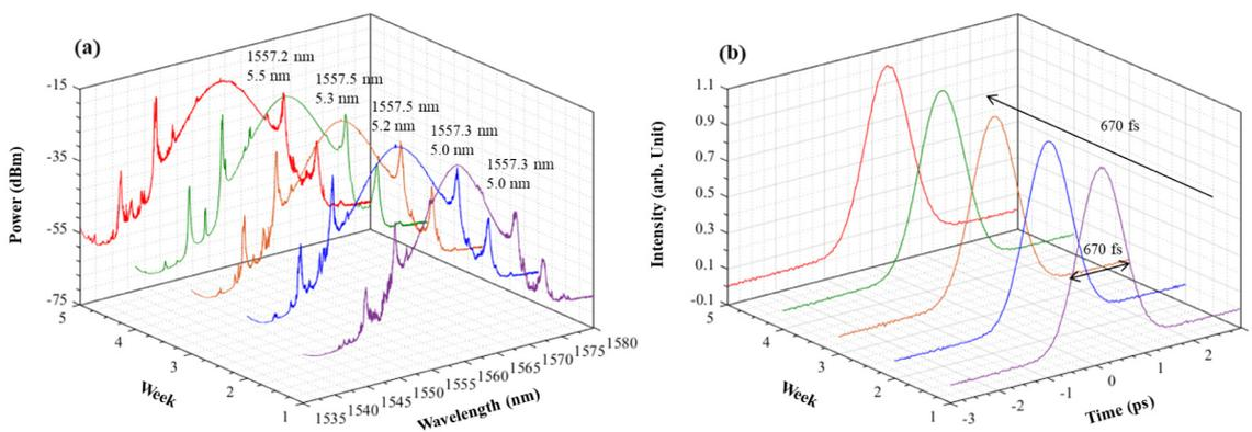
Fig. 4. Sustainability evaluation of (a) optical spectrum and (b) autocorrelation trace of MLFL for four consecutive observation weeks.
