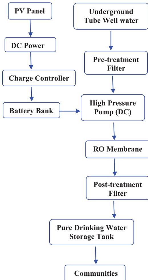
Fig. 1 Block diagram of the pure drinking water system.
