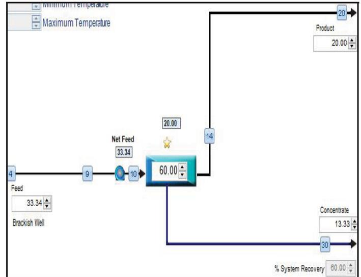
Fig. 5 RO purification system flow diagram
