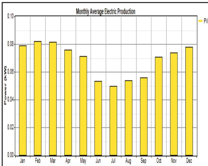
Fig. 6 Monthly electricity production from PV system
