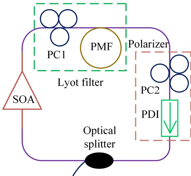
Fig. 1: The experimental setup of MWFL based on IDT mechanism utilizing unidirectional Lyot filter.
