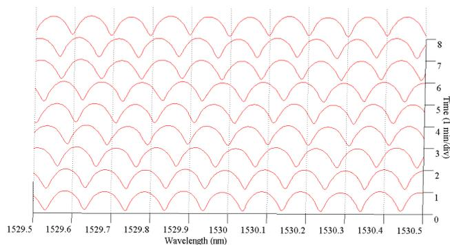
Fig. 5: Wavelength stability of the MWFL spectra within 8 min of interval time.
