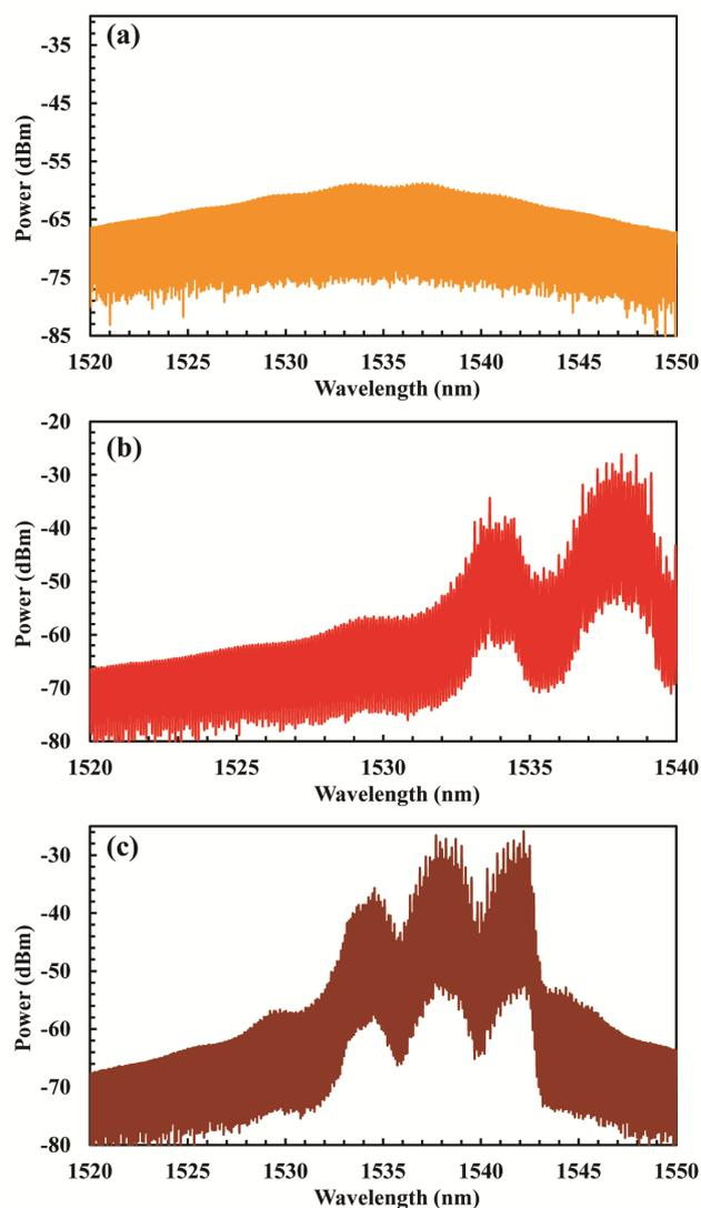
Fig. 4. Multiwavelength spectra based on throughput port of 90% when the SOA current is set to (a) 100 mA, (b) 150 mA and (c) 200 mA.
