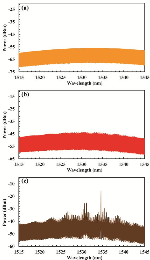
Fig. 3. Multiwavelength spectra based on throughput port of 10% when the SOA current is set to (a) 100 mA, (b) 150 mA and (c) 200 mA.
