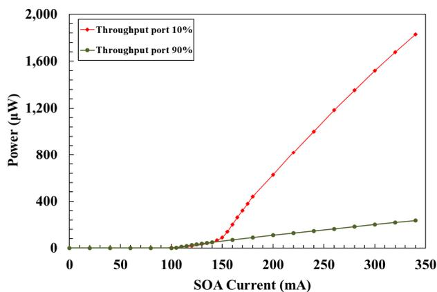
Fig. 2: The lasing threshold comparison of the best performance of MWFL based on different throughput port variation.
