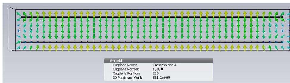
**Figure 3.** Plot of 2D Electric field between the copper plates where the direction of the vertical field is downward as shown by the green arrows. This is because the top plate was defined to have positive surface charge density (+Q) while the bottom plate has negative surface charge density (-Q). The fringing effect could be seen clearly at the both edges of the plot
