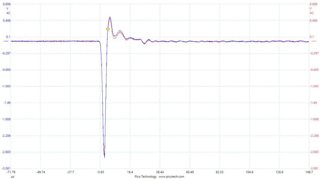
**Figure 8.** An example of captured waveform of +NBE flash. The blue plot is signal captured by metal plate antenna system and the red plot is signal captured by FR4 copper plate antenna system
