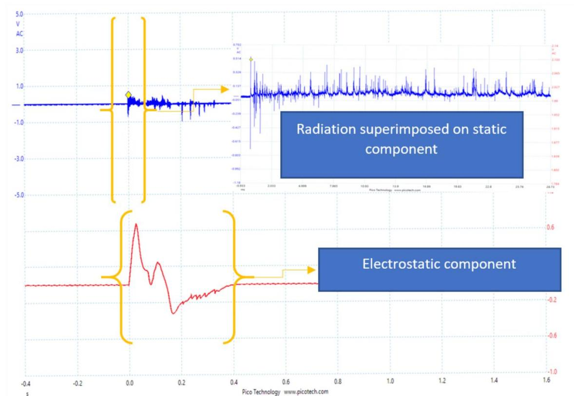
**Figure 12.** An example of IC flash captured with radiation component superimposed on static component (top blue plot) and electrostatic component (bottom red plot)
