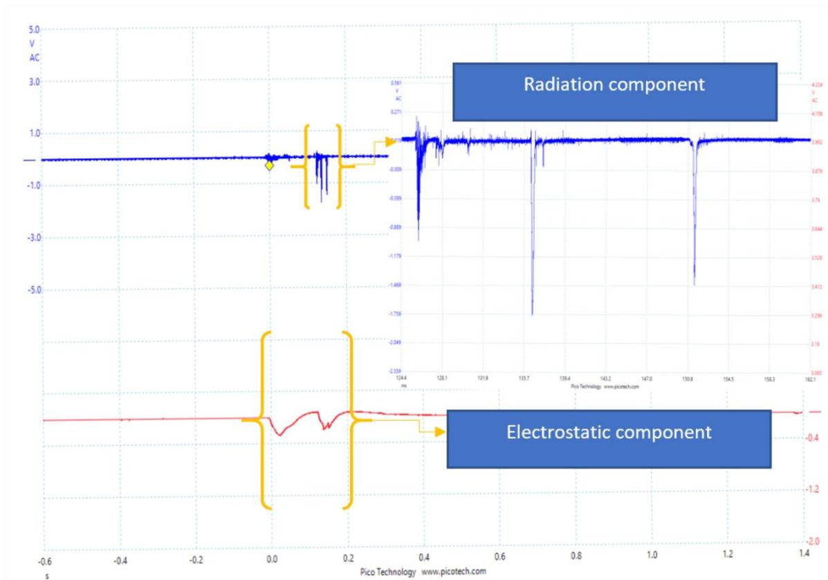
**Figure 10.** An example of IC flash captured with radiation component (top blue plot) and electrostatic component (bottom red plot)
