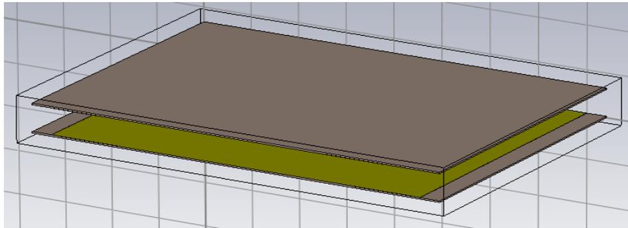
**Figure 1.** Model of a parallel plate with thin copper plates facing each other and separated by 3 cm air gap
