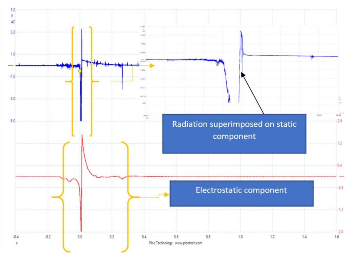
**Figure 11.** An example of  $-CG$  flash captured with radiation component superimposed on static component (top blue plot) and electrostatic component (bottom red plot)
