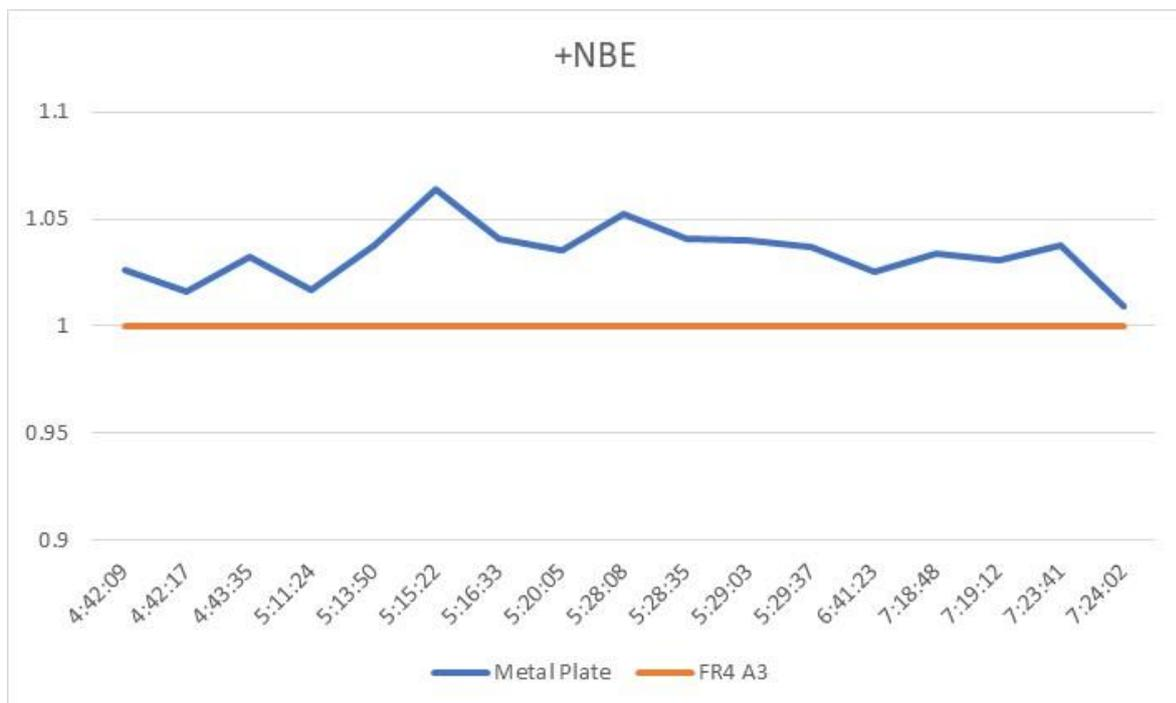
**Figure 6.** Plot shows the performance comparison between metal plate antenna and FR4 copper plate antenna for +NBE flashes. The ratios are determined based on peak electric field values of metal plate over the values of FR4 antenna
