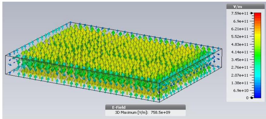
**Figure 2.** Plot of 3D Electric field between the copper plates. It is clear that the electric field is almost uniform between the plates (green arrows) except at the edges due to fringing effect
