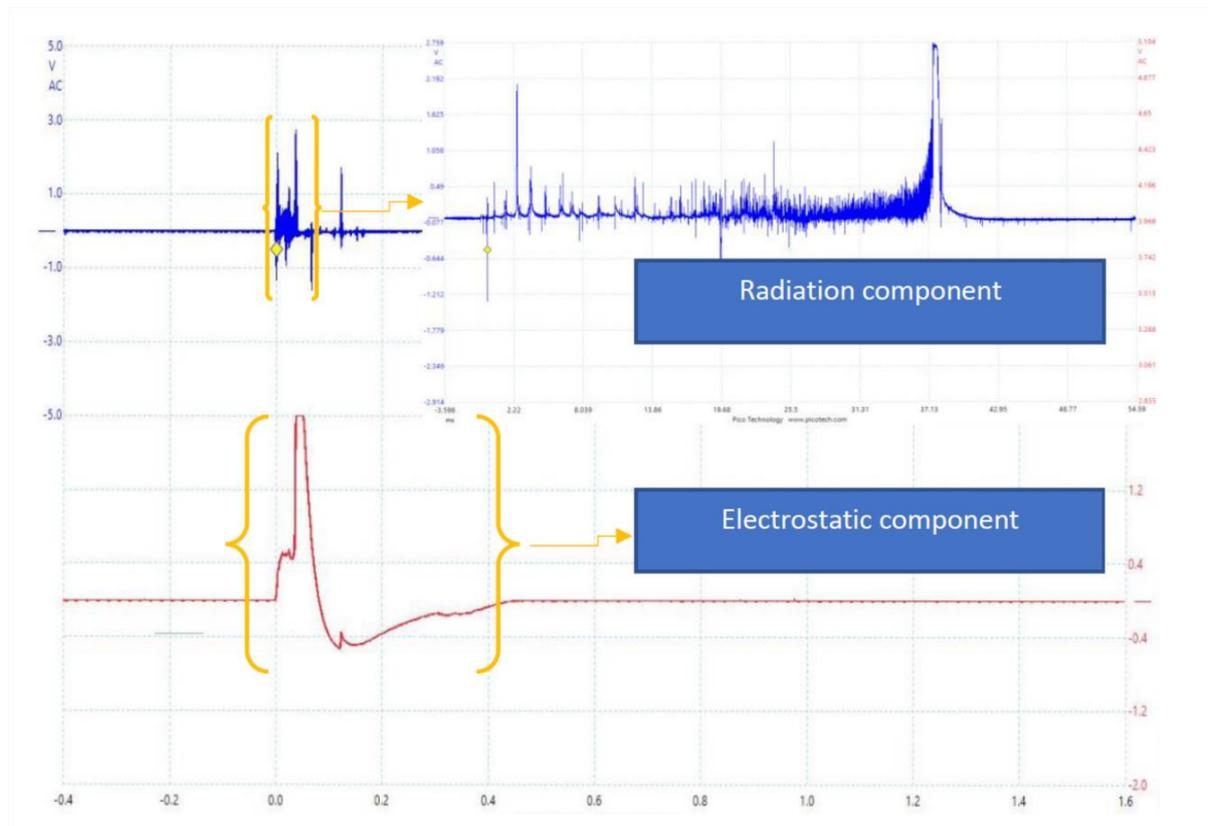
**Figure 9.** An example of  $-CG$  flash captured with radiation component (top blue plot) and electrostatic component (bottom red plot)
