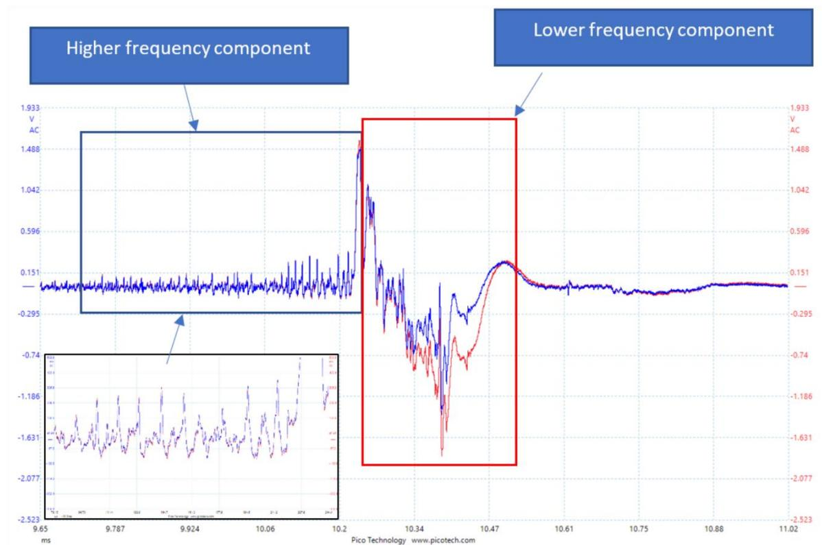
**Figure 7.** An example of captured waveform of  $-CG$  flash that consists of stepped leader and return stroke processes. The blue plot is signal captured by metal plate antenna system and the red plot is signal captured by FR4 copper plate antenna system
