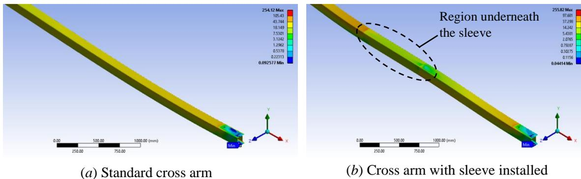
**Figure 4.** Comparison of stress contours of first (outer) cross arm composite layer between both cases.
