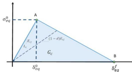
**Figure 1.** Damage initiation and propagation points.
