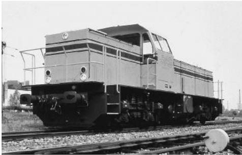
Fig. 9.16: Diesel-electric locomotive DE 1003 of RAG (Bombardier Transp.)
