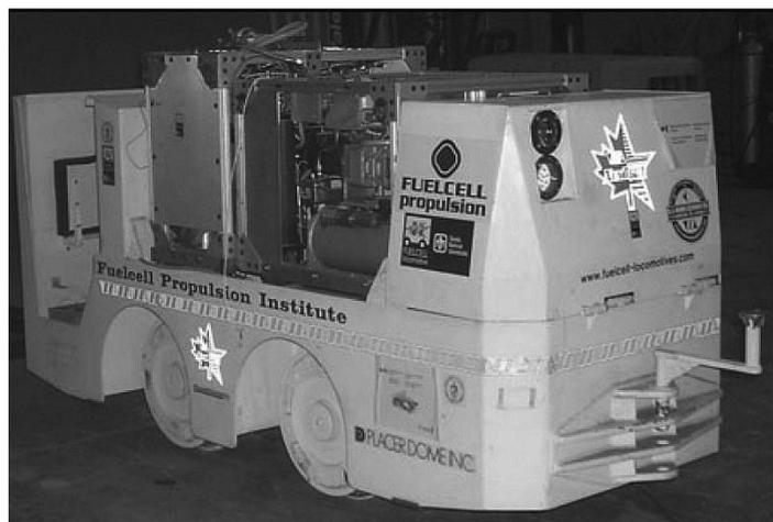
Fig. 10.29: Mining locomotive prototype with PEM fuel-cell stack ([www.fuelcellpropulsion.org](http://www.fuelcellpropulsion.org))
