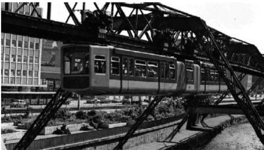
*Fig. 12.6: Wuppertal suspension railway*
