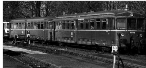
Fig. 10.28b: Accumulator motor coach ETA 150 of DB (1953-57)
