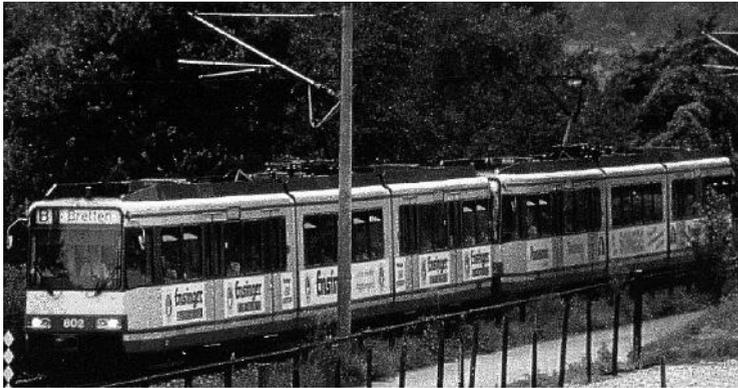
Fig. 10.12: Dual system Light Rapid Transit train GT8-100C/2S on 15-kV, 16 <sup>2</sup>/<sub>3</sub> -Hz line (Bombardier Transportation)
