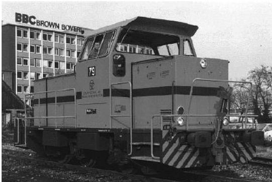
Fig. 9.9: Diesel-electric shunt locomotive DE 501RAG
