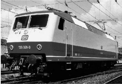
Fig. 1.9: Full-electric high-performance locomotive class 120 of DB; 1979, 5600 kW
