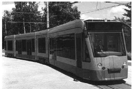
Fig. 10.23: 100 % low-floor multi-joint tram Combino (DÜWAG-Siemens)
