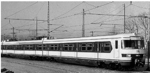
Fig. 10.4: Metro train Class 420 DB (Bombardier Transportation)
