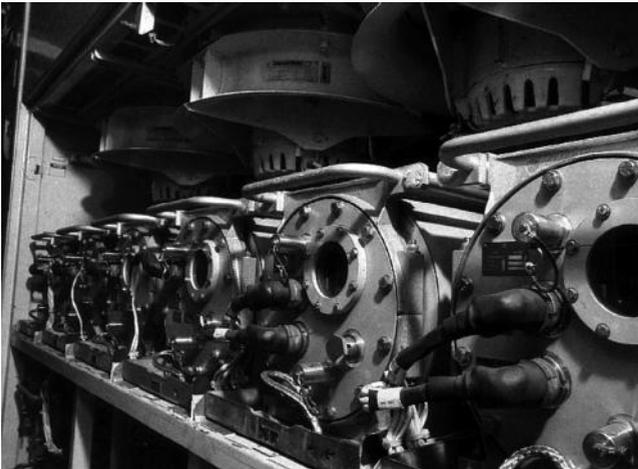
*Fig. 7.10: Evaporative-cooled thyristor converters of TGV-A (Alstom Transports)*
