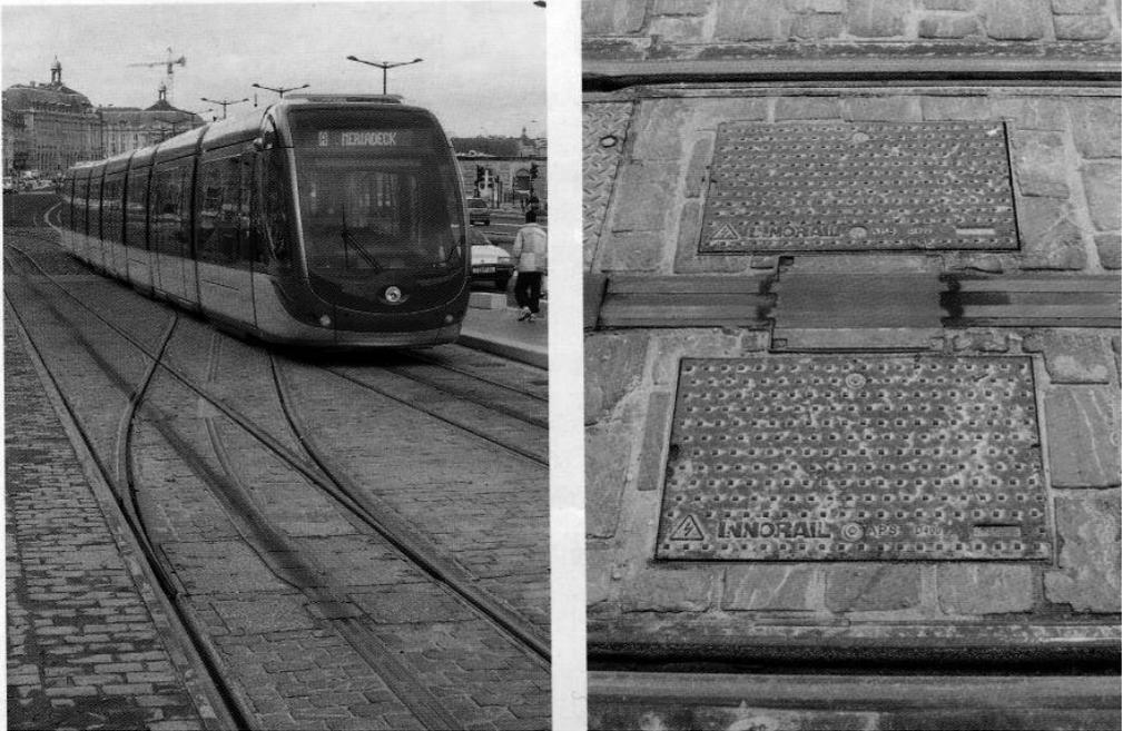
Fig. 13.28: Bordeaux APS tram (CITADIS) and power-enabling switches between the rails
