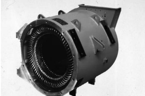
left: Stator with casing
