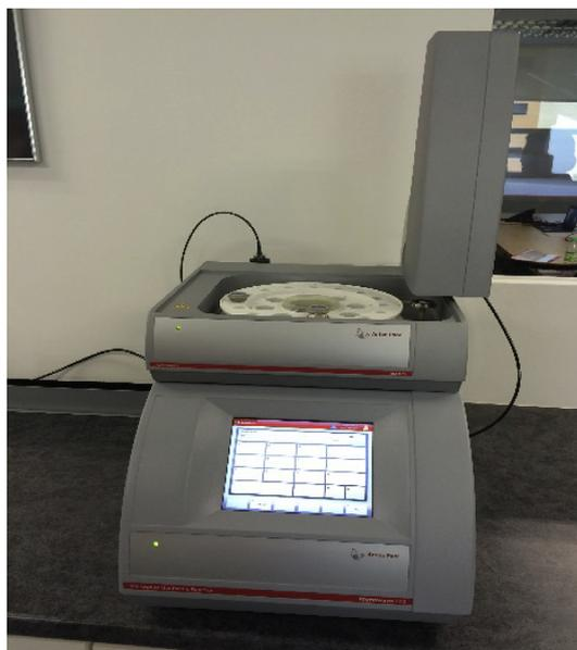
Fig. 1. Anton Paar Monowave 400 microwave reactor.
