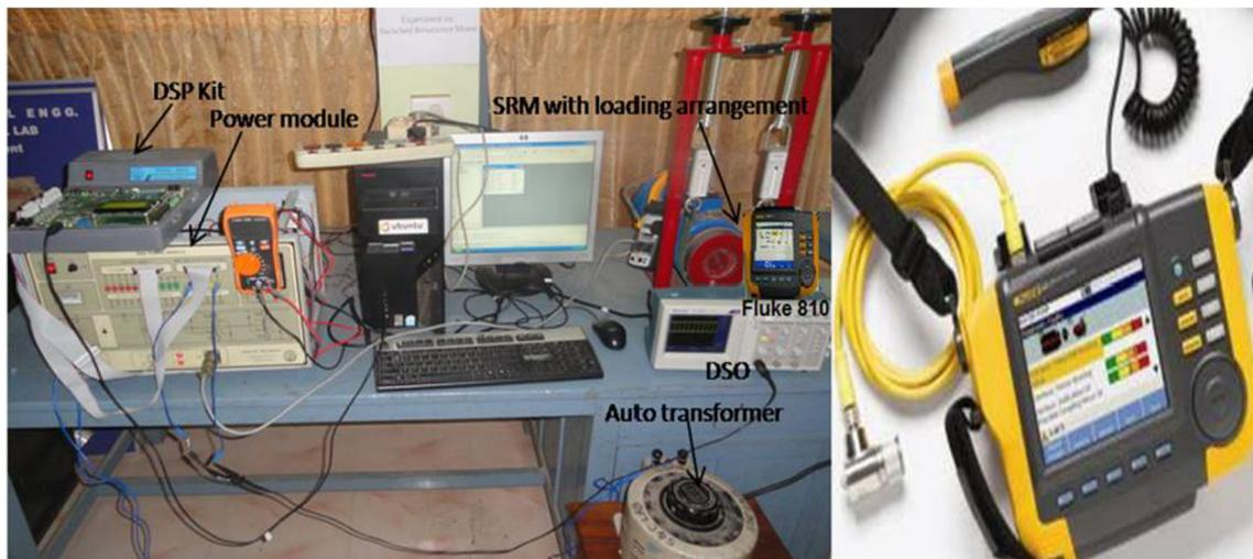
Fig. 12 Experimental setup of vibration measurement using Fluke 810 Vibration Tester
