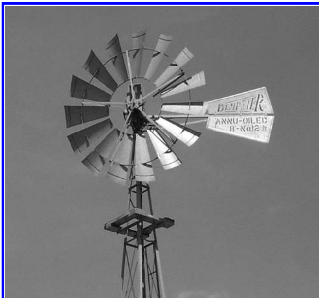
FIGURE 43.2 Typical American multiblade windmill. (Courtesy of Nolan Clark, U.S. Department of Agriculture.)
