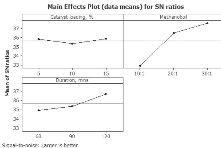
**FIGURE 2.** Main effects plots for ‘larger-is-better’ SN ratio analysis of each parameter.
