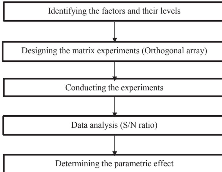
**FIGURE 1.** The Taguchi design process flow-diagram
